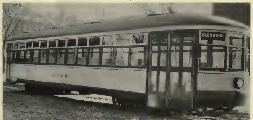
One of the light-weight, noiseless type cars put in operation by the Twin City Rapid Transit Company
