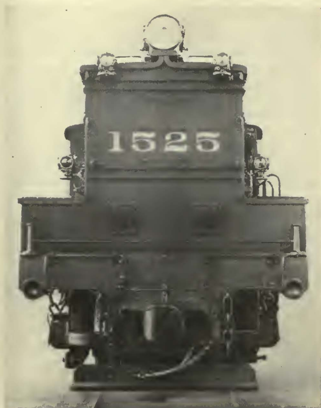
The battery sections are narrow enough to permit an unobstructed view by the engineer
