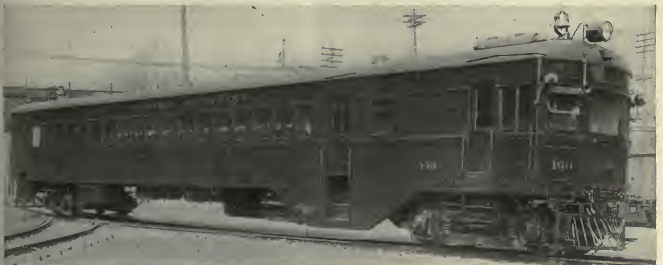
A typical 73-ft., 250-hp. Brill-Westinghouse gas-electric car of the Boston & Maine Railroad
