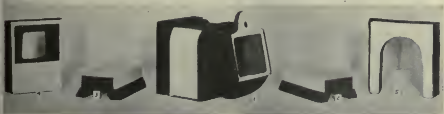
1. Journal box with chilled surface painted white. 2 and 3. Chills used in pedestals.
