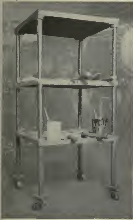
Convenient material rack for the electrical repair department
