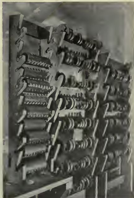
Storing cylinders in this neat and systematic manner has improved the shop appearance and lessened the possibility of mechanical injury prior to installation
