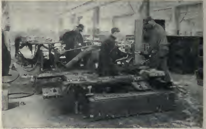
At left—Heating rivets in a portable fuel oil forge alongside the work At right—Riveting new manganese wear plates to truck pedestals
