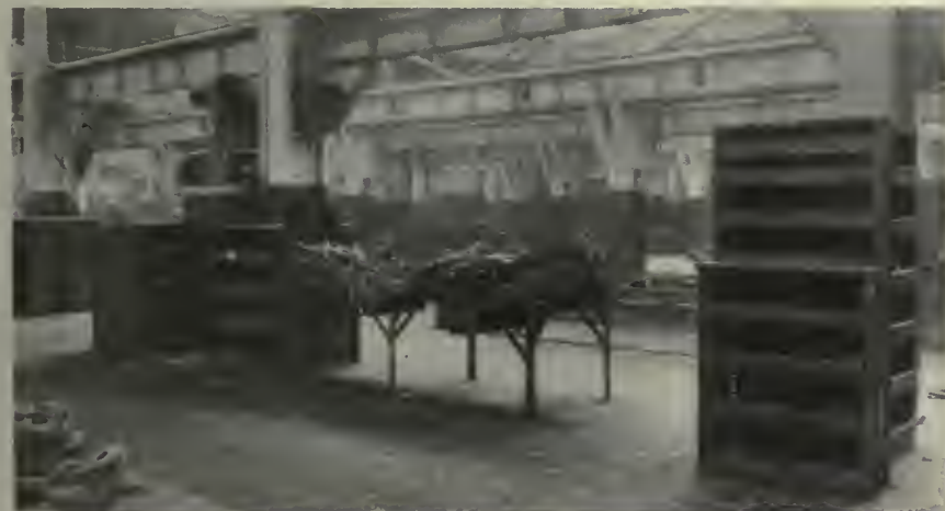
Free stores are located immediately adjacent to the truck overhauling section. Small parts are kept in bins and larger parts in racks
