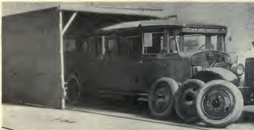
Portable shed used in Grand Avenue shops of the Connecticut Company to speed up process of bus painting
