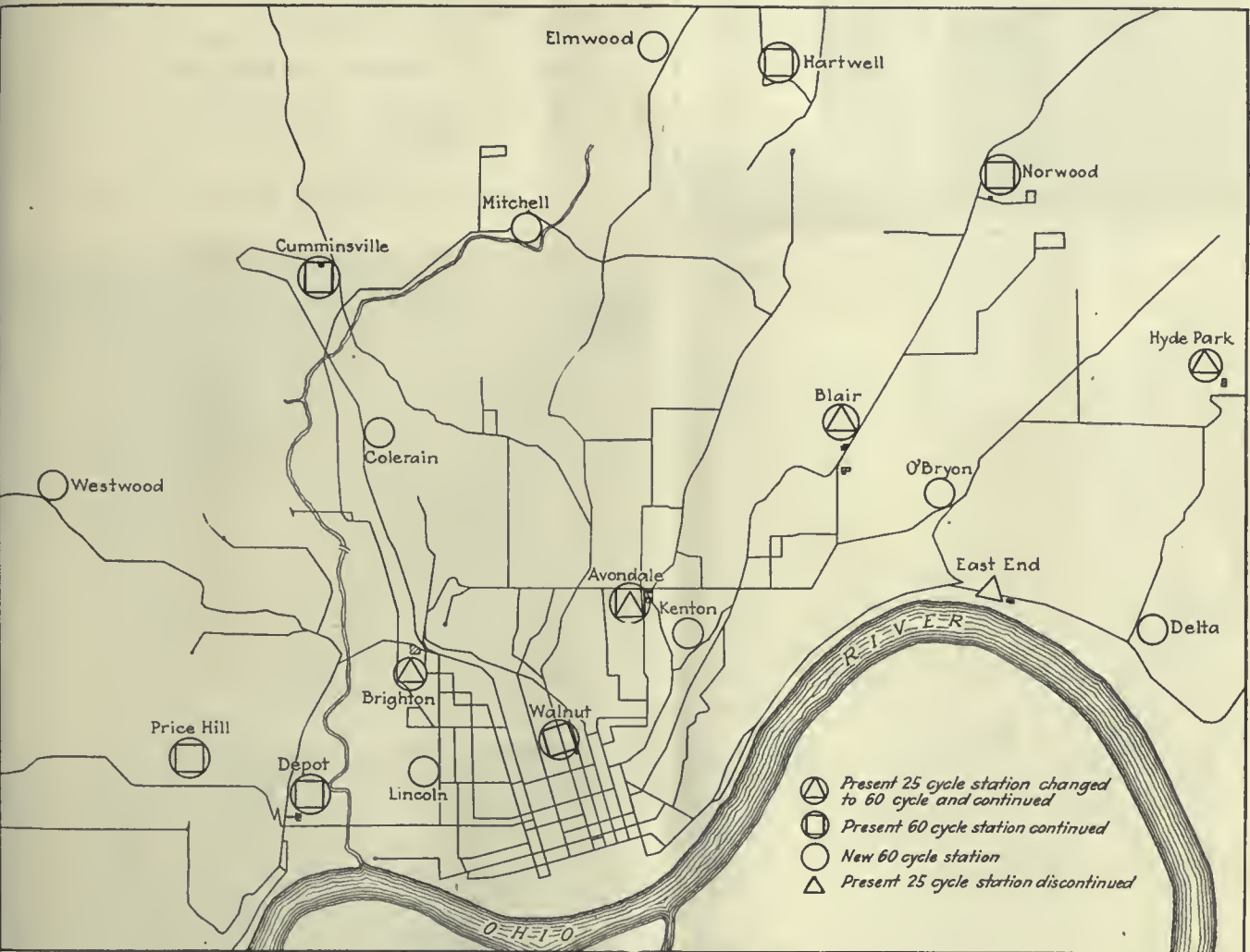
New power distribution system of the Cincinnati Street Railway
