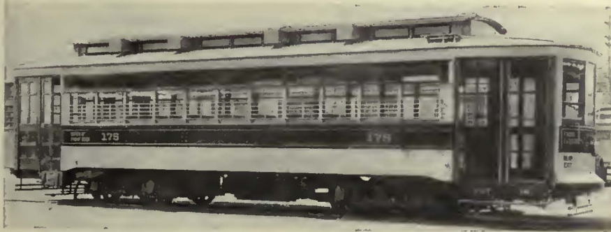
One of the double end, one-man cars recently delivered to the Washington Railway & Electric Company
