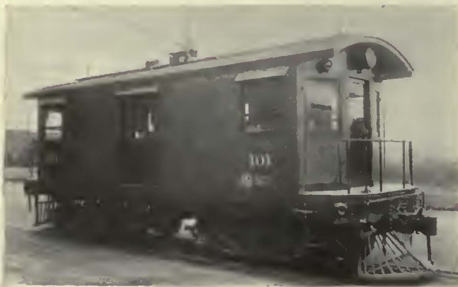
Locomotive of the Alabama Power Company used in belt-line freight service in Tuscaloosa, Ala.
