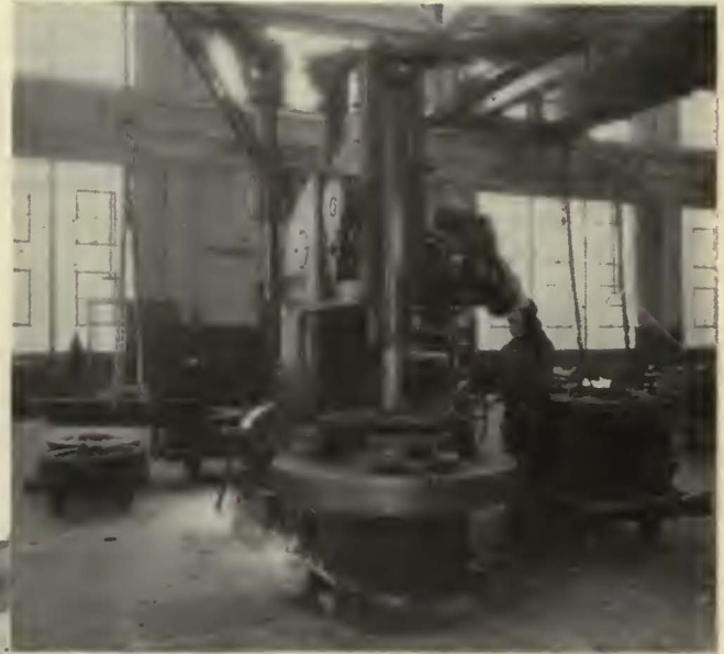
At top—Boring out a subway wheel. The wheel suspended from the crane on the left is ready to be swung into position. A truck at the right receives wheels after they are bored. The crane at the right handles finished wheels
