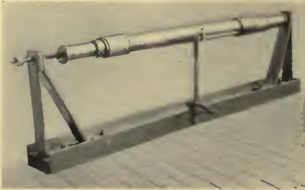
Testing an axle for eccentricity by means of a jig made in the Norfolk shop of the Virginia Electric & Power Company
