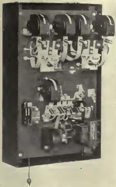
Mechanism of starter removed from case
