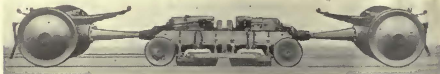
Early Zurich radial axle truck for Cardan drive
