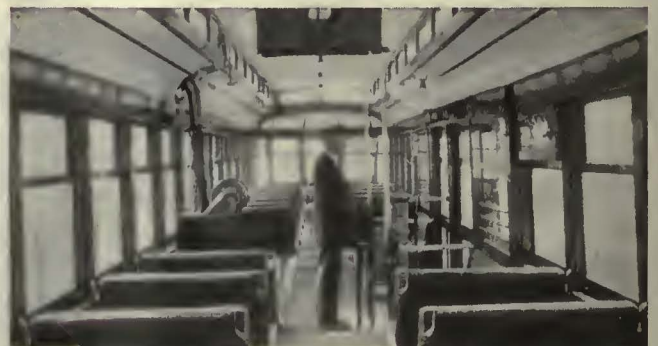
Longitudinal seats have been replaced by leather upholstered cross-seats in this Detroit trail car
