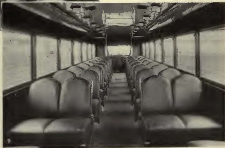
Leather-upholstered, deep spring-cushioned seats insure passenger comfort. The car is arranged for double-end operation. Note the overhead rail handholds in the corners of the body
