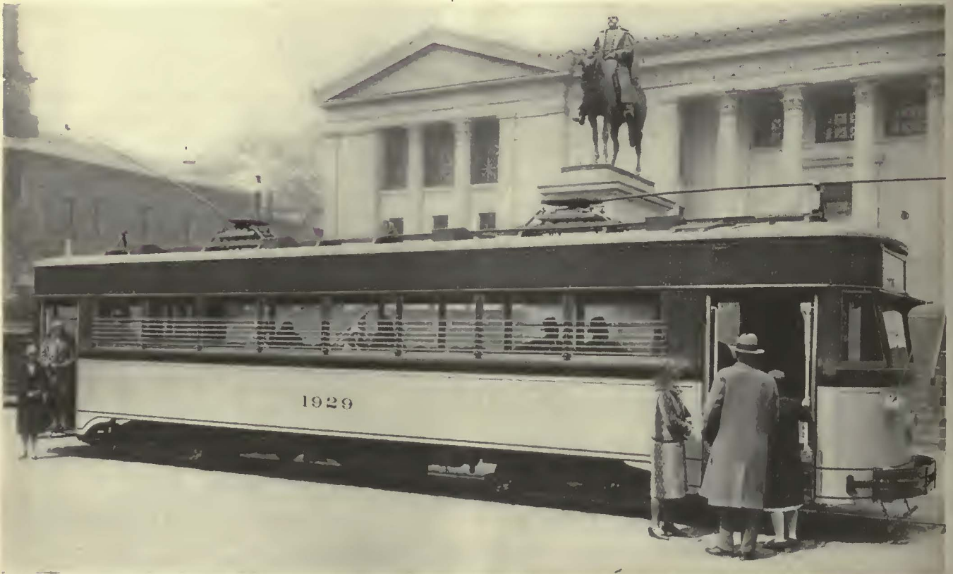
Sample car designed by Osgood-Bradley Car Company to meet 1929 transportation conditions. No attempt was made to achieve extreme light weight, but special attention was given to the proportions and appearance of the body
