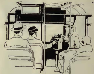
The indication of the National Fare Register is visible to passengers in the car.
