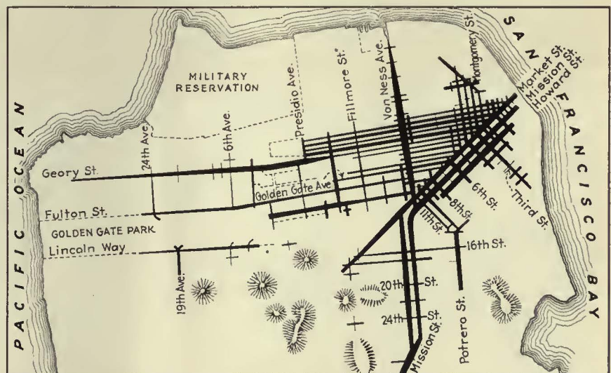
Relative vehicular traffic load on principal traffic arteries of San Francisco, based on an eight-hour count, from 8 a.m. to 12 noon, and from 2 p.m. to 6 p.m., September, October and November, 1926
