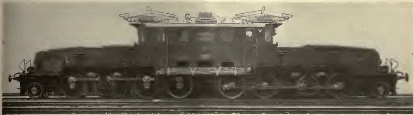
Mountain type high-speed passenger locomotive of 1100 series used by the Austrian State Railways
