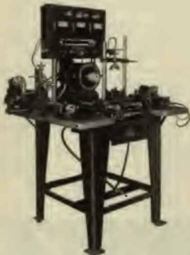
Heavy-duty test bench for bus electrical equipment
