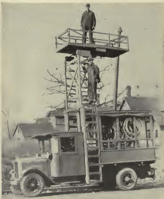
The platform of this Twin City Rapid Transit tower truck is raised and lowered hydraulically by a power take-off on the transmission
