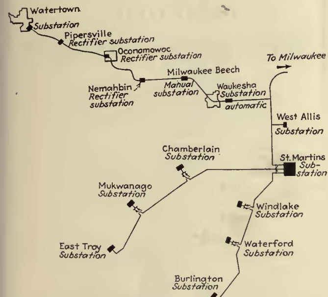
Pipersville, Oconomowoc and Nemahbin rectifier stations are located on the Milwaukee-Watertown interurban line, while Chamberlain, Wind Lake and Waterford rotary-converter substations supply power to the East Troy and Burlington lines
