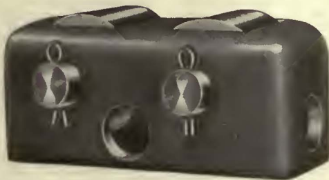
In this side bearing the rollers are large and the parts are chromium plated
