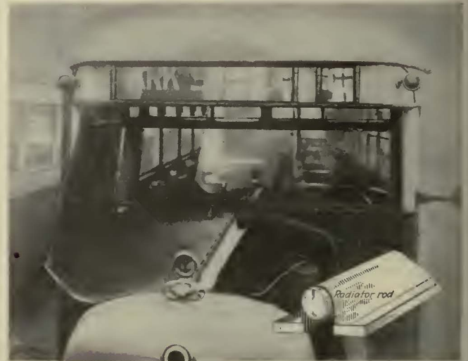
The rain trough is made of ordinary light-weight sheet metal, so shaped as to fit snugly over the radiator tie rod and slope sufficiently toward the rear to lead all water away from the ignition circuits
