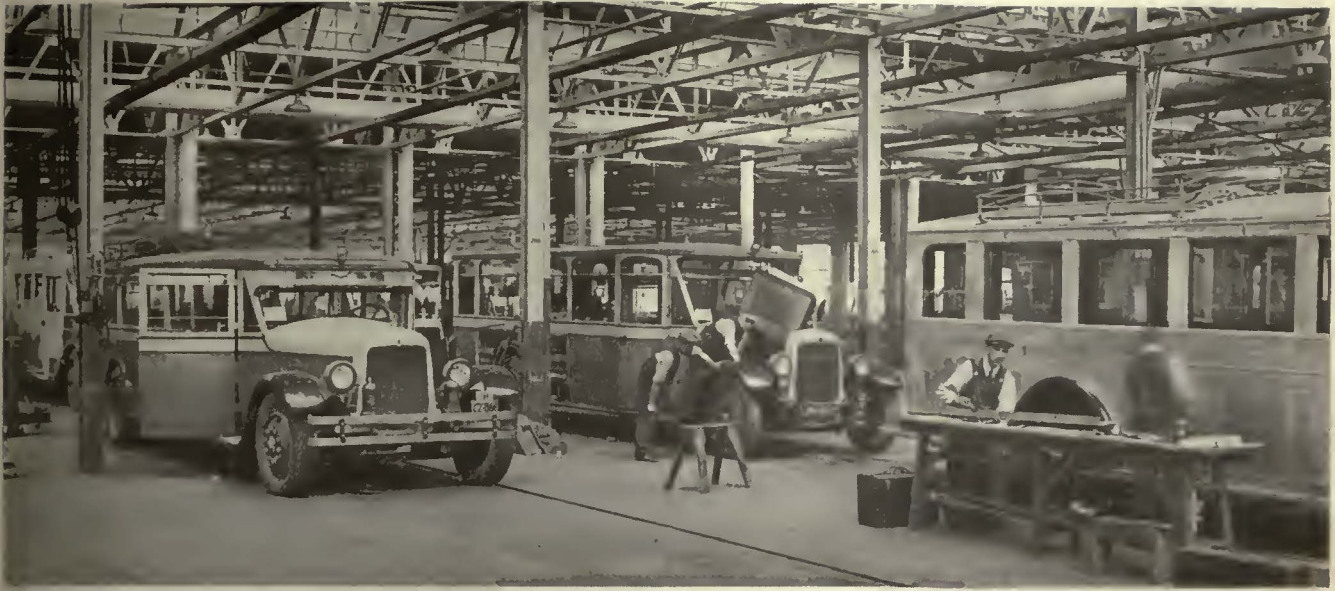
Overhauling bus bodies at the Hillcrest general shops of the Toronto Transportation Commission
