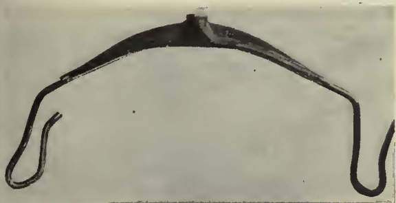
A new 00 trolley ear, 12 to 15 in. long, usually withstands 1,000 lb. dead load as this one did. Note the central holding section continues to surround the wire, while the approach ends are slightly loose
