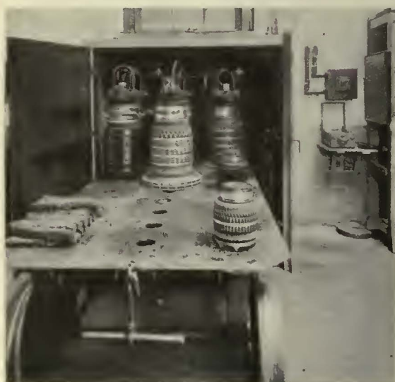
At left, armatures are tested during baking at shop of New Orleans Public Service, Inc. At right, connections for insulation test equipment
