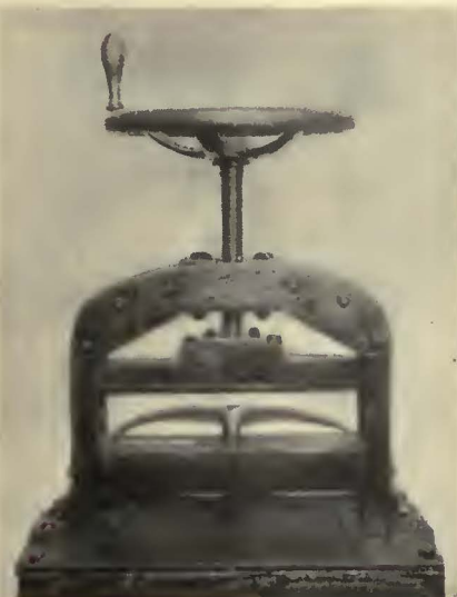
At right, trolley ear in press for reclaiming. At left, straightened ear after the pressing operation
