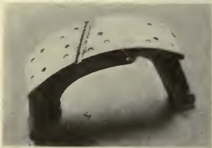
A diagonal groove cut across the face of the brake lining supplies an outlet for dirt particles that ordinarily would be ground into its surface
