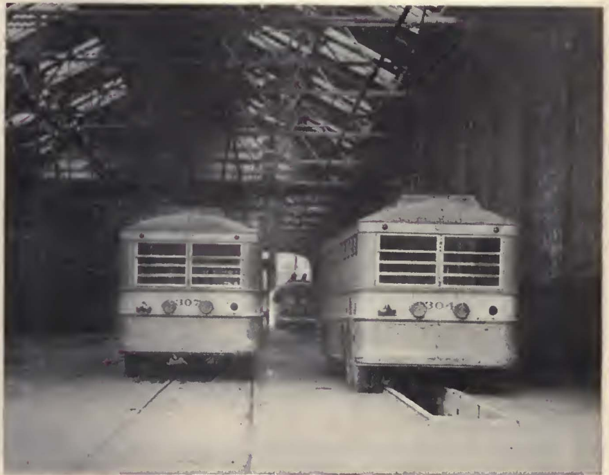
Carhouse pits were readily adapted at small cost to meet the needs of electric coach inspection and maintenance
