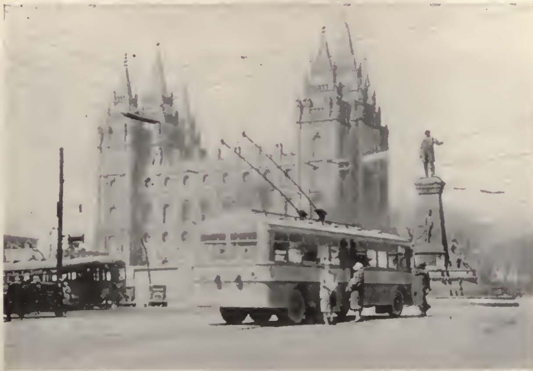
Ten electric coaches of this type, manufactured by the Versare Corporation and equipped with Westinghouse motors and control, are operated on the Salt Lake City route
