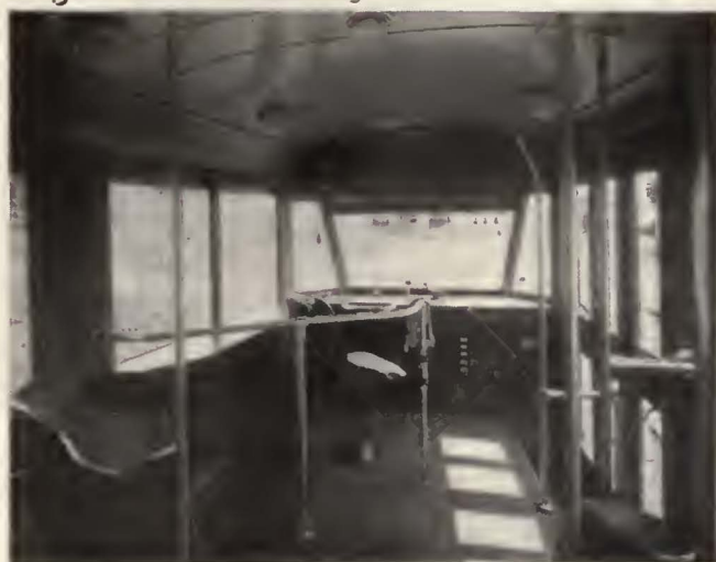
All control equipment is encased in a cabinet
