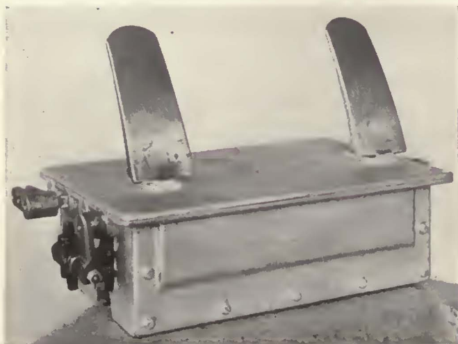
This pedal control for power and brake is mounted in a recess on the cabinet
