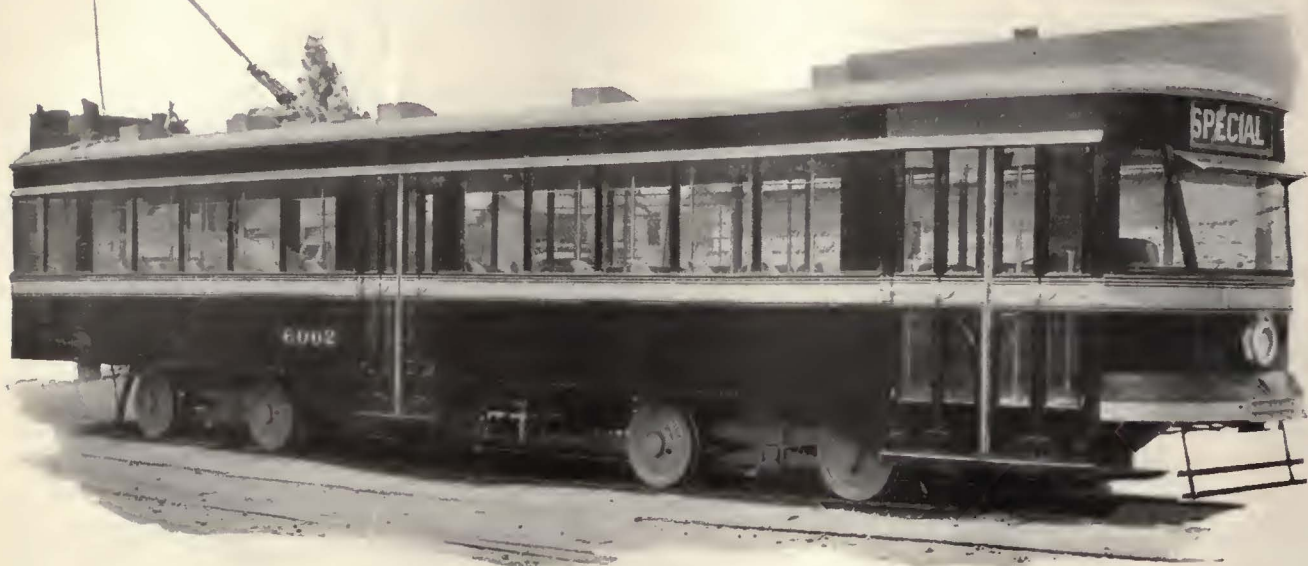
While the new Pittsburgh car resembles those built last year it weighs 27,000 lb. as compared with 36,500 lb. for the earlier model and the exit is at the center instead of the rear
