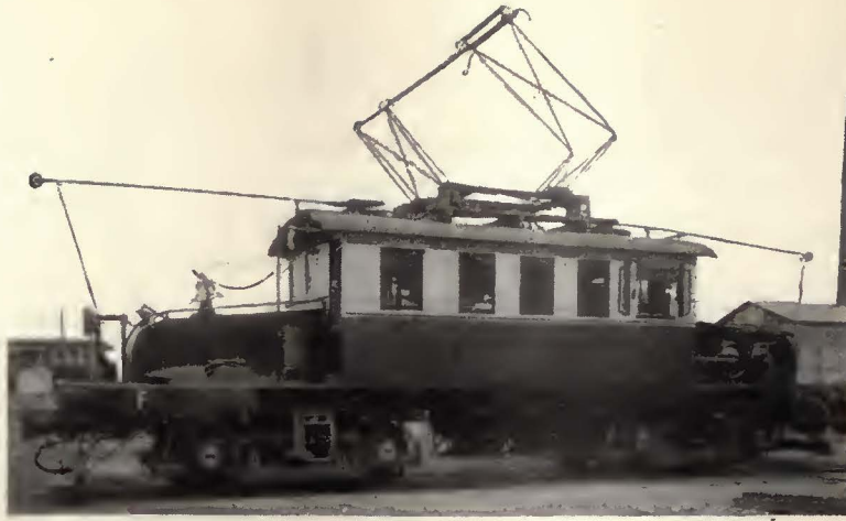
One of the new 600-hp. electric freight locomotives equipped for either pantograph or trolley operation
