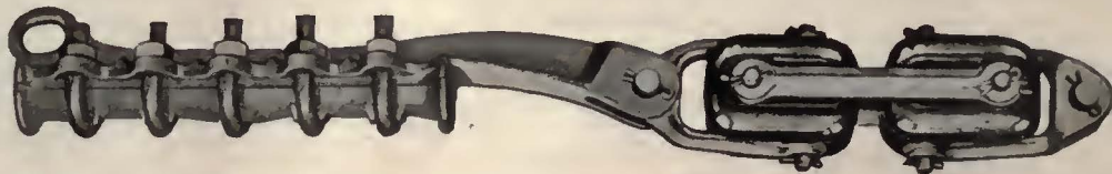
O-B Feeder Dead End Clamp Assembly for use with feeder cables of any size from 4-0 to 1,000,000 c.m. inclusive. Clamps and fittings are of Flecto iron. Insulators, O-B XH strain insulators. Page 2, Supplement No. 2 to Catalog No. 20.
