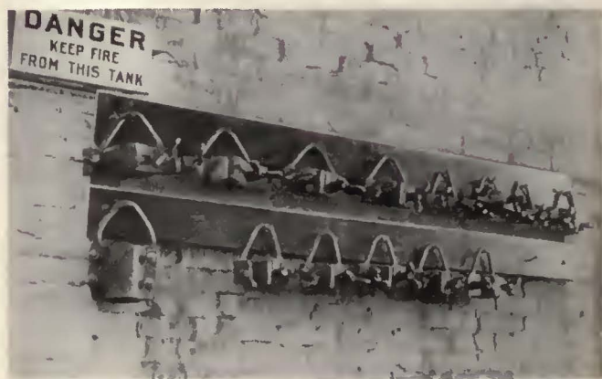
Armature shaft clamps of various sizes are neatly stored on a rack located directly above varnish vats
