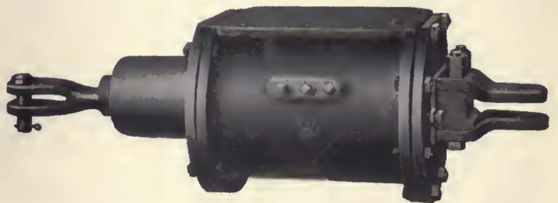
The brake cylinder is the business end of your brake system and should be large enough to develop sufficient shoe pressure with a leverage ratio low enough to assure proper shoe clearance.
