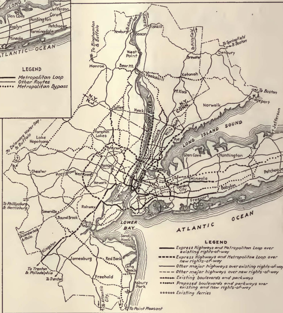
Diagrammatic scheme of highway routes. This plan includes a highway loop, a roughly rectangular system of routes within the loop, and circumferential, radial and connecting routes. The actual application of this scheme to the contours and present development of the land with the greatest feasible usage of existing highways is shown below
