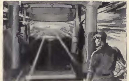
The coning press forms the web of the wheel to the proper curvature or "cone." This is the last of the "hot" operations.
