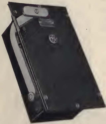
The foot-operated master controller of the PCM-equipped car leaves the operator's hands free
