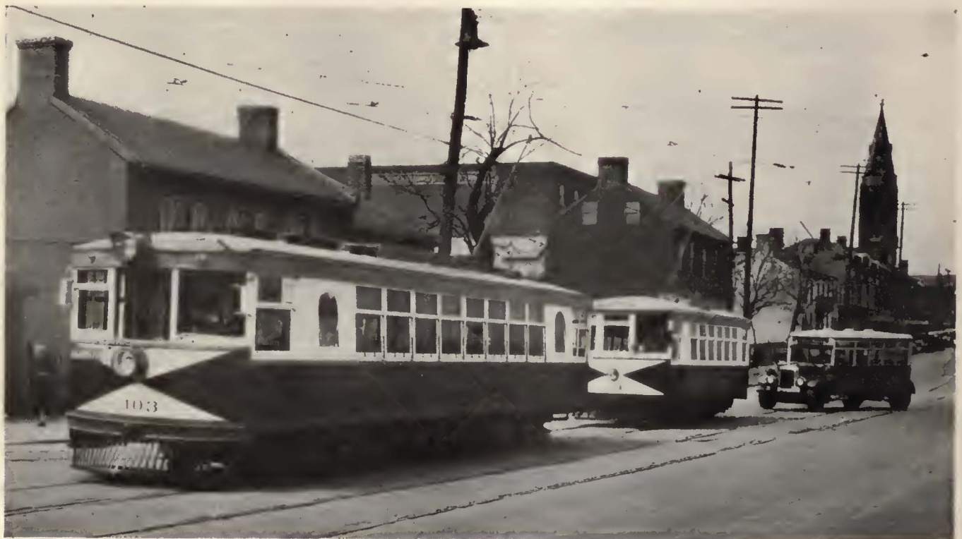
Twelve light-weight double-truck interurban cars and 27 single truck city cars replaced all of the equipment formerly in service. This represented an investment of $306,999. In addition, a modern bus service was developed to replace former jitneys
