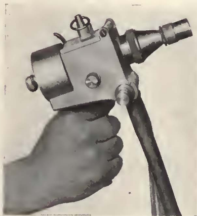
Metal in wire form fed into this gun may be sprayed on any metal or non-metallic material
