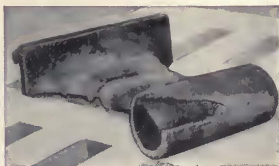
Cast-iron support for a drill table on which carbon paste is used to hold welding metal
