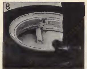
Applying Tire 4—Continue walking around rim.
