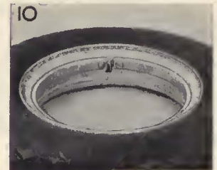
Tire on Rim—Ready for inflating and mounting on wheel.
