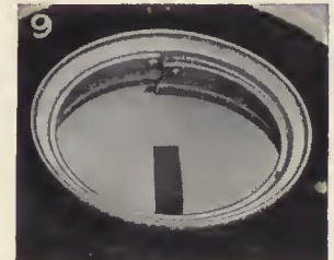
Applying Tire 5—Close rim by dropping on block or with gentle blow from a 2- to 4-pound hammer.
