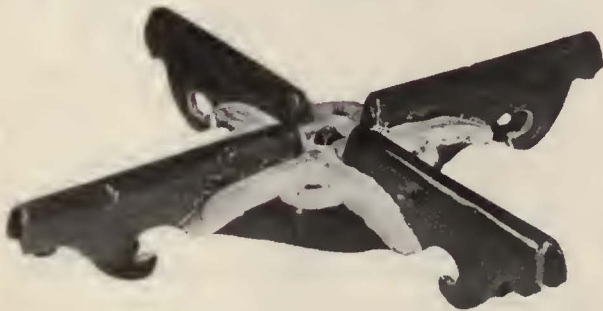
The 90 deg. overhead crossovers were redesigned to accommodate the sliding plate bow collectors by filling in the clearance gap somewhat and leveling the leads
