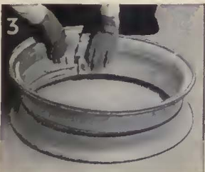
Closing Rim 1—Match valve notches in rim parts. Grasp and spread as shown. Hook end of split section on ring.
