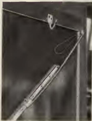
V-shaped hook which holds window wiper off glass when not in use
