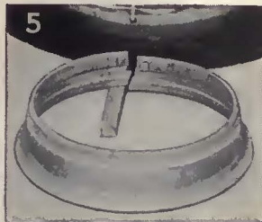
Applying Tire 1—Rest rim section on a 2-inch block as shown. Apply tire, valve pointing upward.
