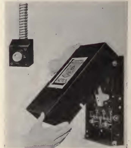
Starting switch and push-button control
