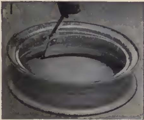
Opening Rim 1—Insert tool in notch near split. Push downward and toward center of rim.
