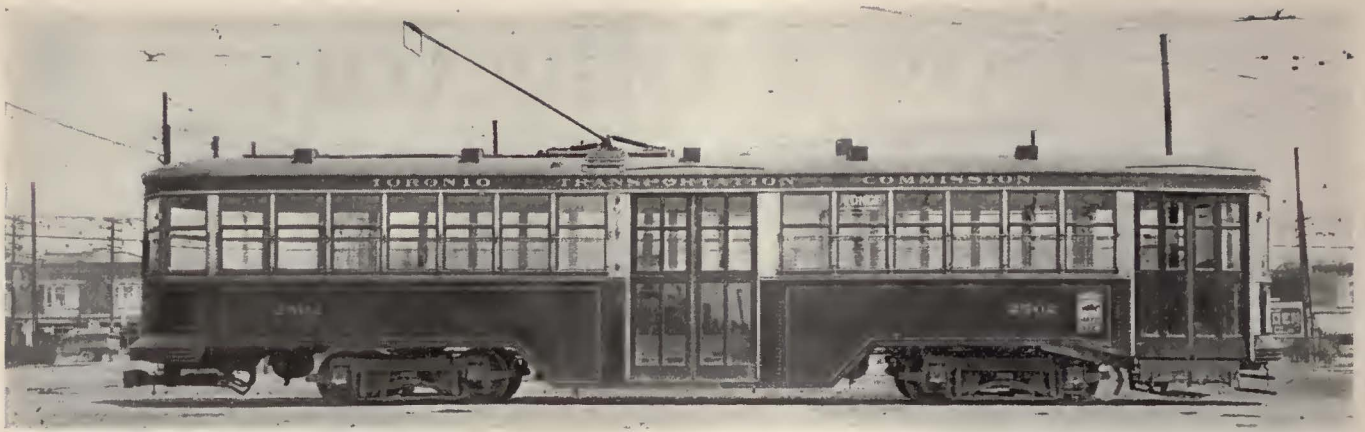
Several cars on the Yonge Street line are equipped with the type of sliding plate collector illustrated
