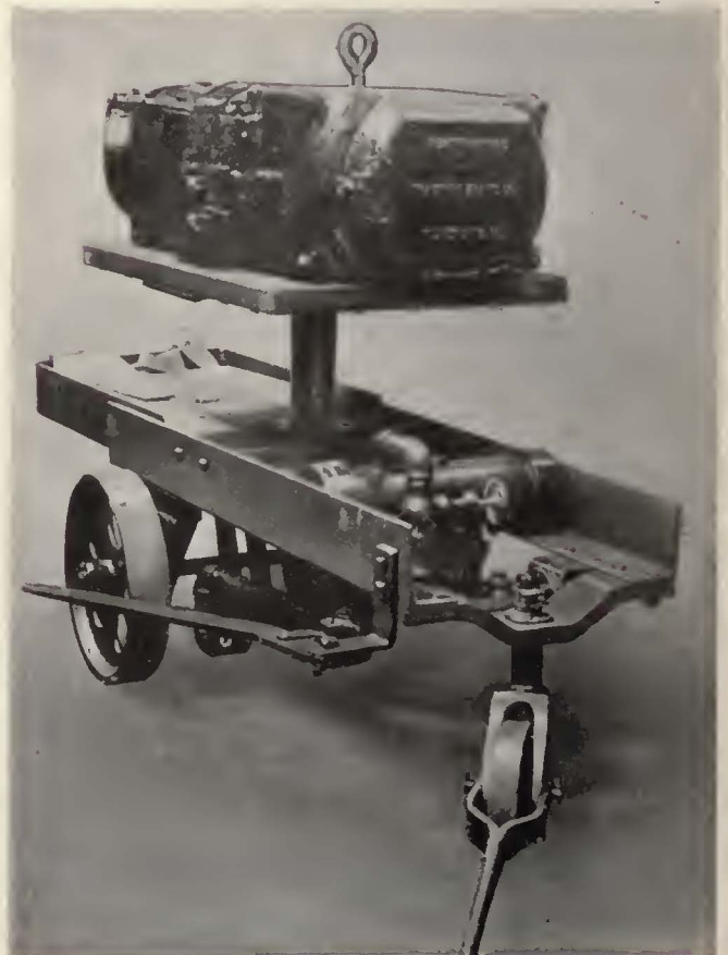
Hydraulic lift for heavy units in use by the Kansas City Public Service Company
