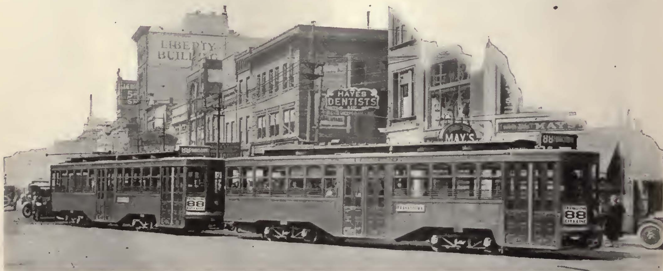
Multiple-unit cars provide a convenient means of handling light traffic during the day and heavy traffic in the rush hours
