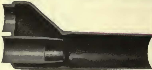
The Vac-Vent Ejector, the heart of the system. Exhaust gases from the motor in leaving the jet, create a powerful suction in the surrounding chamber. This is the operating force upon which the Vac-Vent system depends. A vacuum pressure of two pounds is often produced.
