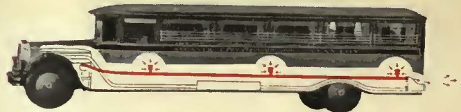
The suction pipe connects with dome-shaped ventilating heads in the floor of the bus, drawing out the foul, cold air, and causing efficient circulation of warm, fresh air without drafts.
