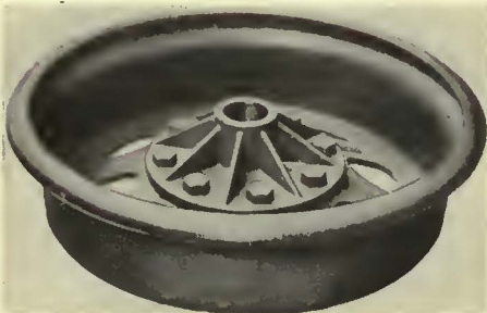
Fairmont demountable wheel of 16-in. rim can be exchanged rapidly if worn out
