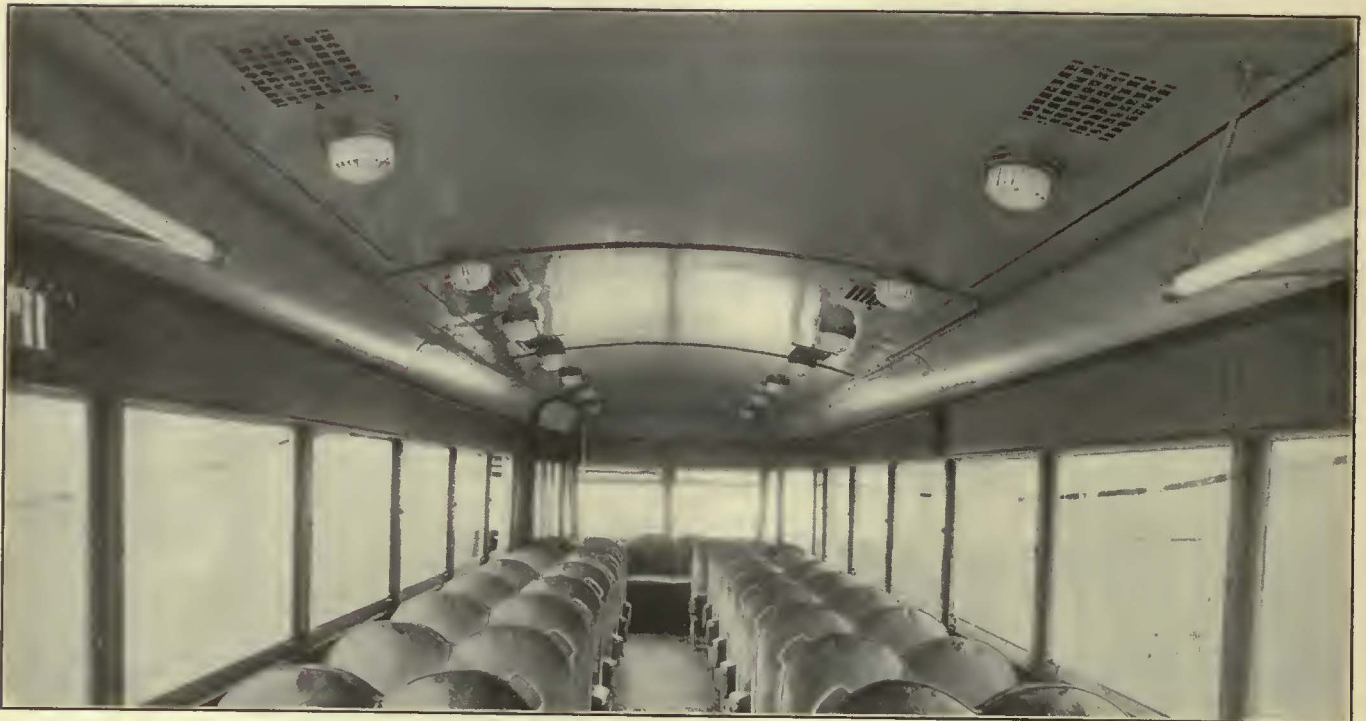
Installation of Type T-twenty-in-series lighting fixtures in a new model Brill Car.
