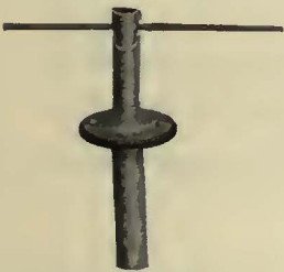
Screw-Type Electrode Holder—A twist of the handle opens and closes it.
