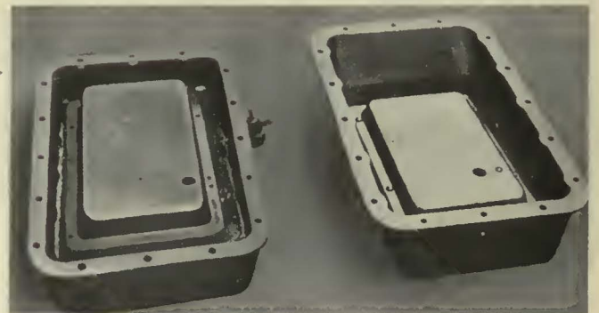
Deeper crankcase eliminates the necessity of replenishing oil supply of the bus at mid-day
