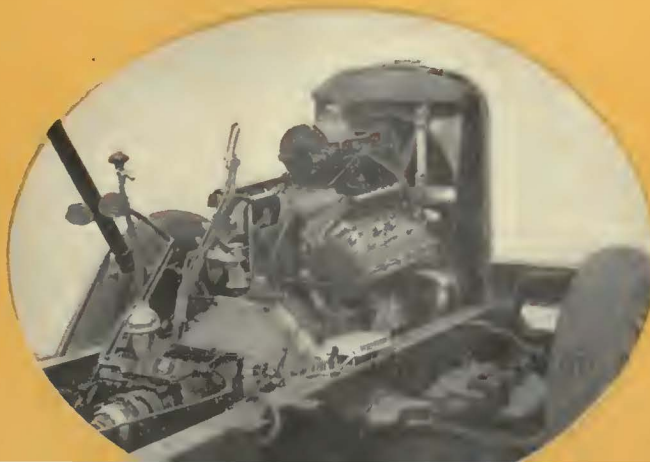
Equipped with the new and more powerful 8 cylinder, V-Type Cadillac Engine
