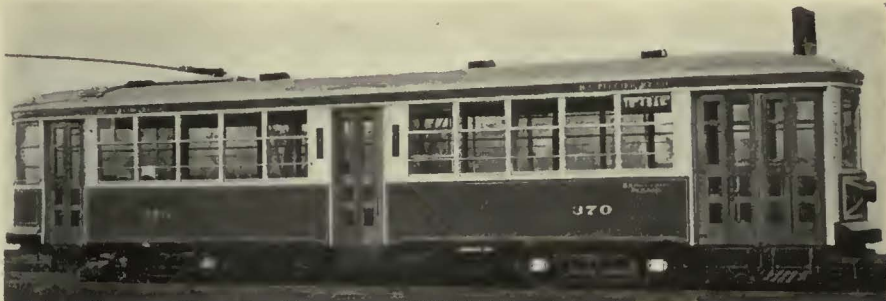
Side elevation of cars recently delivered to the British Columbia Electric Railway, showing unusual arrangement of exit doors
