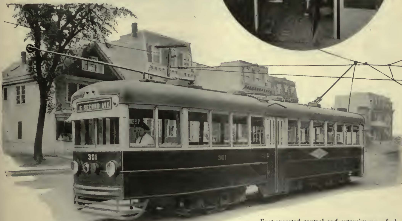
Foot-operated control and extensive use of aluminum in the framing are features of this new car for the United Traction Company of Albany, N. Y.
