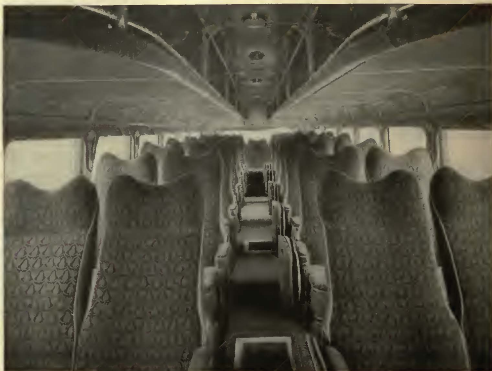
29 permanent seats with six auxiliary folding aisle chairs and tilt seat at right of driver bring total seating capacity up to 36.
