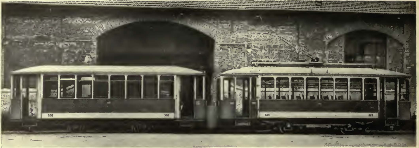
Train service consists of one motor car and trailer, both of the one-truck type. Cars in these trains have all seats facing forward
