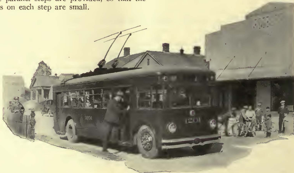
The trolley poles of the coaches are 18 ft. 6 in. in length, permitting a wide range of travel on the streets. In this view the A.C.F. coach has swerved far from the line of the overhead to receive passengers at the curb
