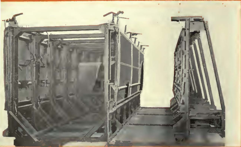
Assembling a side section in a special erection jig. The side panels are of plymstl.
