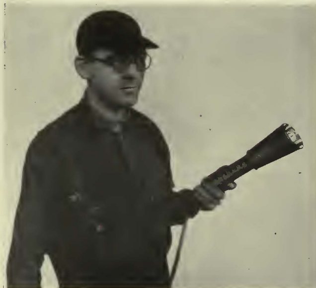
Inspection light used by Cleveland Railway has electrically heated handle
