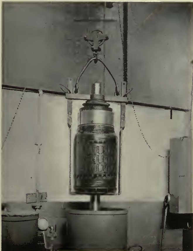
Holder for armatures designed and used by the Dallas Railway and Terminal Company
