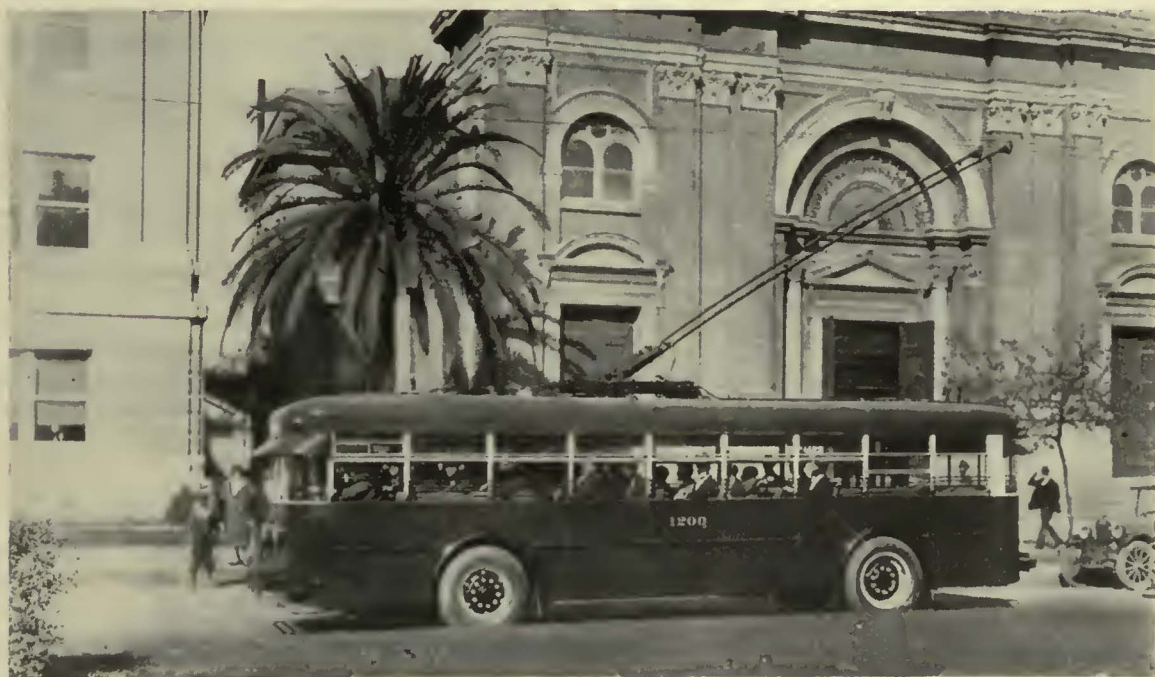
Equipped with two 50-hp. motors each, the New Orleans electric coaches are capable of attaining a maximum speed of approximately 25 m.p.h. and maintaining a schedule speed of more than 10 m.p.h. This view shows the Twin Coach on Carrollton Avenue.
