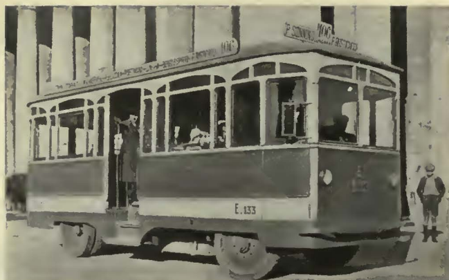
A Lancia bus of the Omicron long type affords seats to 26 passengers and room for 24 standees, and has a rear exit
