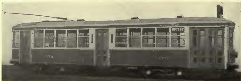
Another Canadian user of aluminum is the British Columbia Electric Railway. Only recently the company received 25 cars of the type shown
