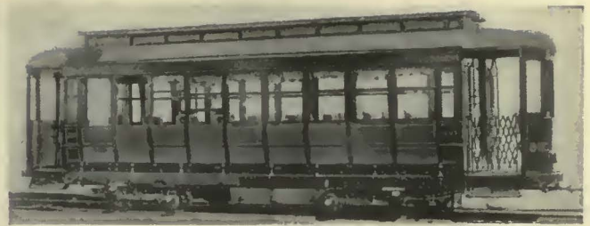
From the vintage of 1905—a car for Manila, using aluminum to withstand the ravages of "white ants"
