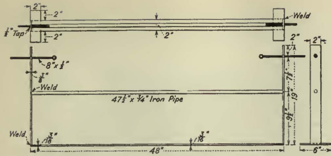
Aligner for wheels has reduced tire wear on buses of the Virginia Electric & Power Company
