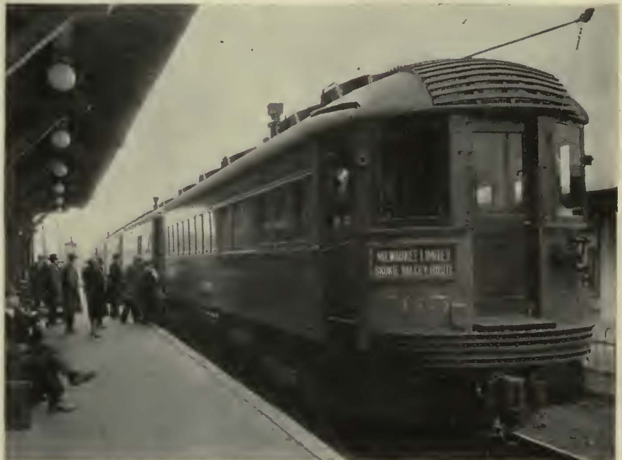
General view of five-car train made up of new all-steel coaches, 25 of which have been placed in limited service on the North Shore Line
