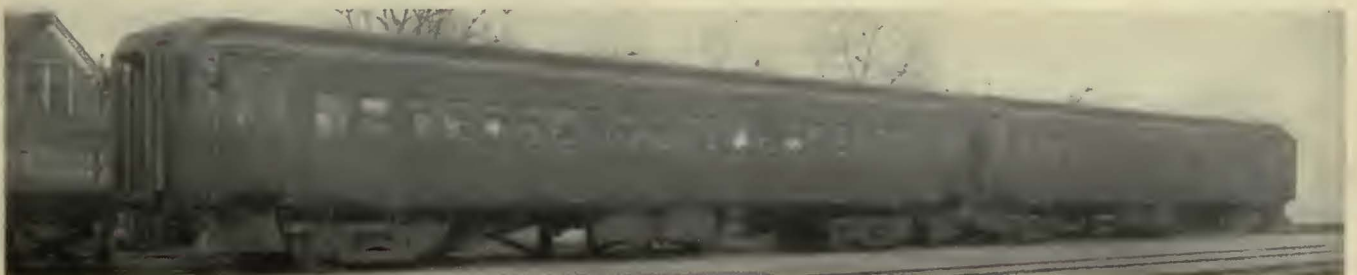
The Illinois Central Railroad pioneered the use of strong aluminum alloys. The two-car train above, one of the first designed, appeared in 1923
