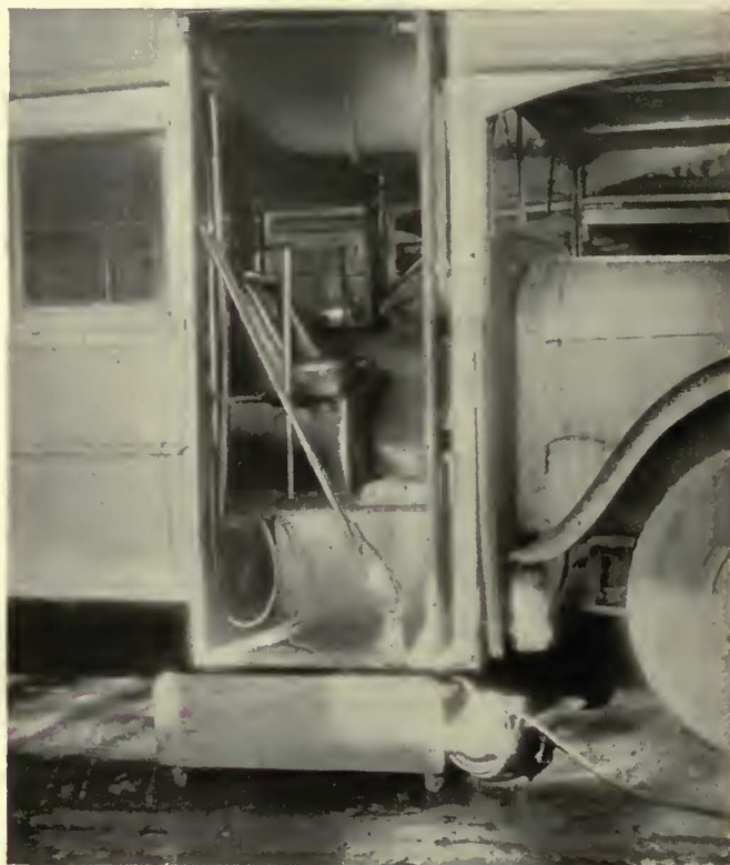
Lighted brooms facilitate sweeping coaches at night in the Cleveland Railway garage
