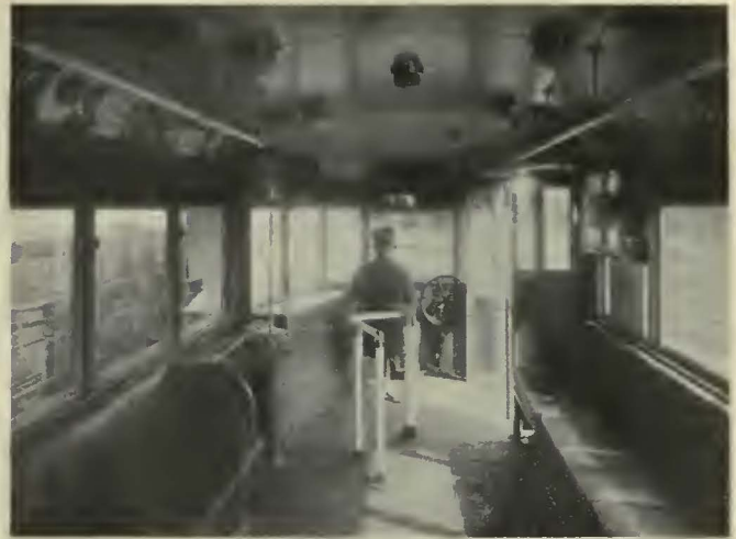
Forward platform of new Brooklyn car, showing motorman's control and arrangement of automatic turnstile at entrance to passenger well
