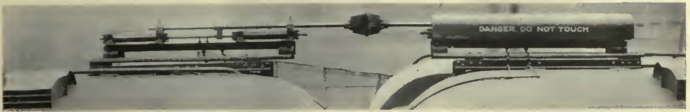
Connectors between cars couple the 11,000-volt train bus lines automatically. This device was designed and developed by the Reading engineers. The cover at the left is removed to show the construction
