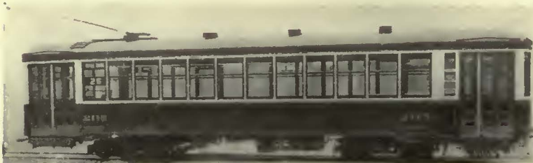
The lighter metal was first used in Canada by the Montreal Tramways. A total of 80 cars with aluminum are now in service on this property
