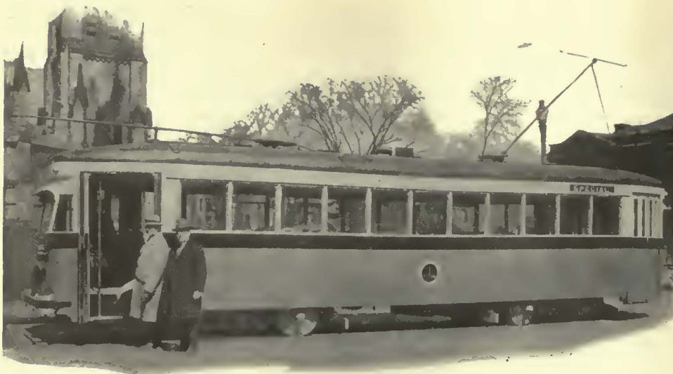
Early in 1927 the Springfield Street Railway introduced its light-weight experimental car, with side members, letterboard and other parts of aluminum
