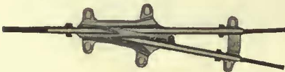
View of pan of O-B Duplex Frog to show overlapping runner construction which increases life of frog and wheel.
