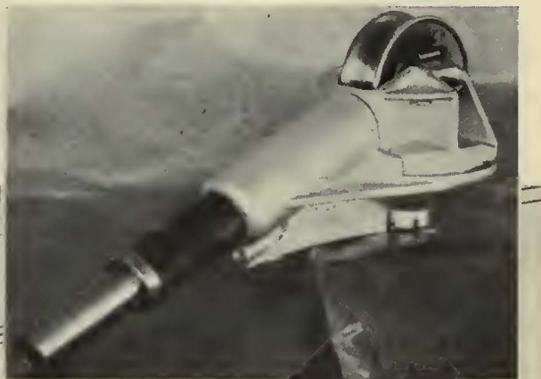
An Ohio Brass swivel harp. The swivel casting is mounted on the lower casting over a 4½-in. ball bearing
