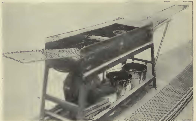
Window guards are painted at a rate of 3\frac{1}{2} sets per hour by one man using this machine in the shops of the Cleveland Railway
