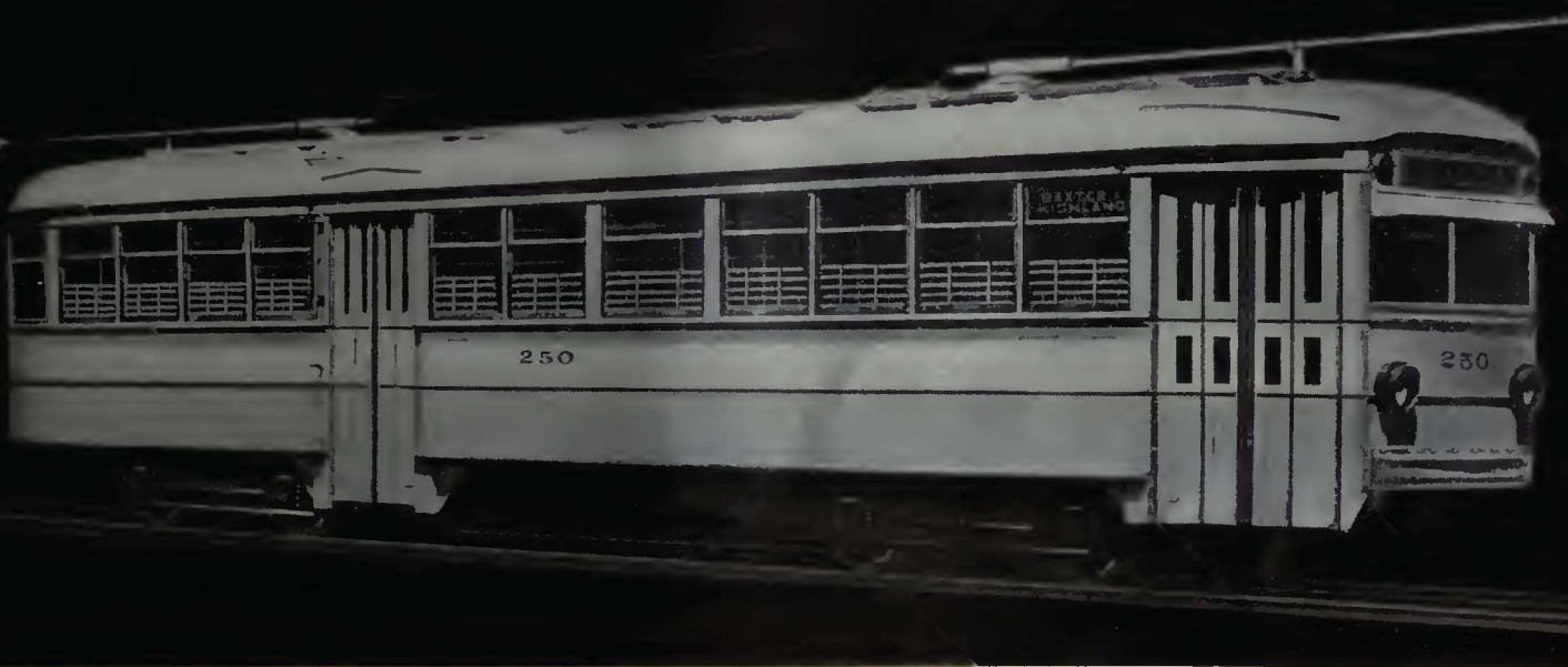
Car built by Cincinnati Car Company for Louisville Railway Company. Structural weight was greatly reduced by use of Alcoa Aluminum and its Alloys.
