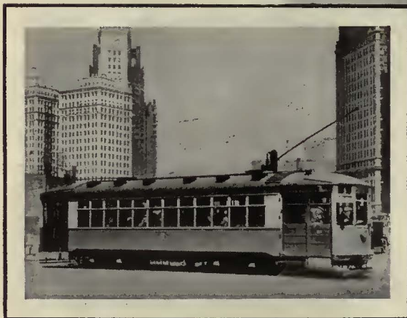
The Chicago Surface Lines specified G-E air brakes and PCM control for 100 new cars. Forty are equipped with GE-301, low-wheel motors.
