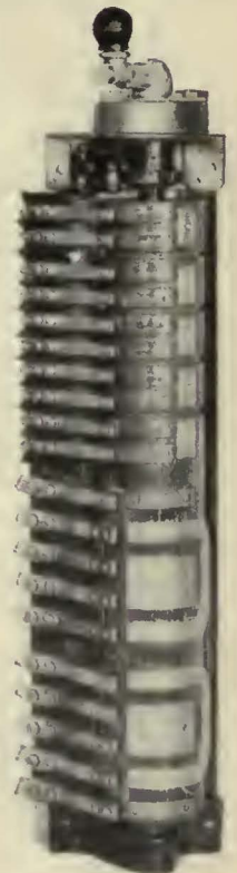
Main control switch group weighing 447 lb. is placed under the floor of the car. Covers are removed in this view. At right—The reverser switch, weighs 42 lb. It is housed in a cabinet at the left of the operator
