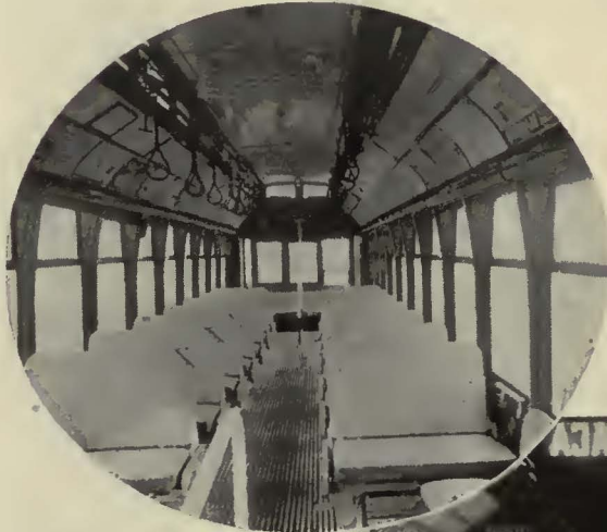
Interior of remodeled Baltimore car, showing fourteen double cross seats, with curved seat on rear platform and longitudinal seat opposite entrance
