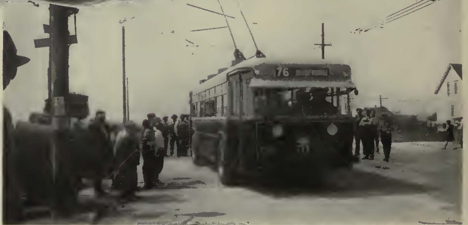
View of new trolley bus for Chicago. Equipment includes O-B Dash-Illuminating Headlights, O-B Featherweight Trolley Bases, O-B Trolley Retrievers, O-B Trolley Poles and the new O-B Swivel Harp and Wheel especially designed for trolley bus service.
