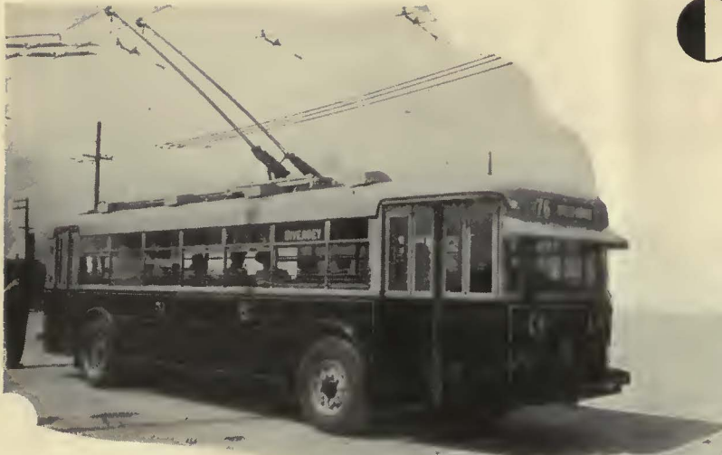
View of new trolley bus for Chicago. Equipment includes O-B Dash-Illuminating Headlights, O-B Featherweight Trolley Bases, O-B Trolley Retrievers, O-B Trolley Poles and the new O-B Swivel Harp and Wheel especially designed for trolley bus service.
