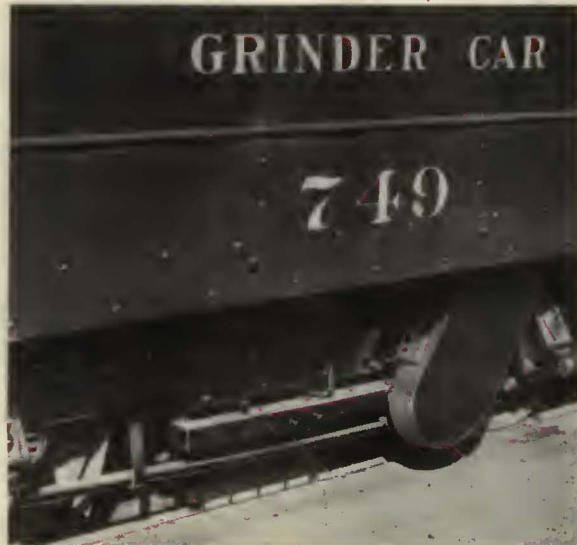
Reciprocating Grinder Car, showing one of the grinding units.
