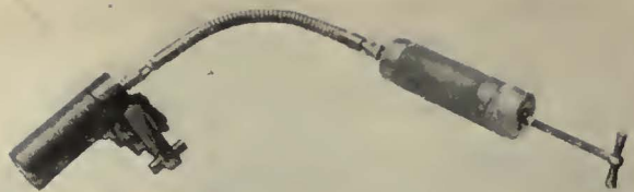
Alemite grease gun for lubricating electric track switches on the Cleveland Railway
