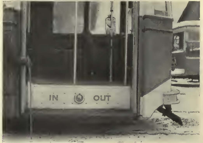
The height of the first step is 13 in. and the second is 12 in. The ramp is 3 in.
