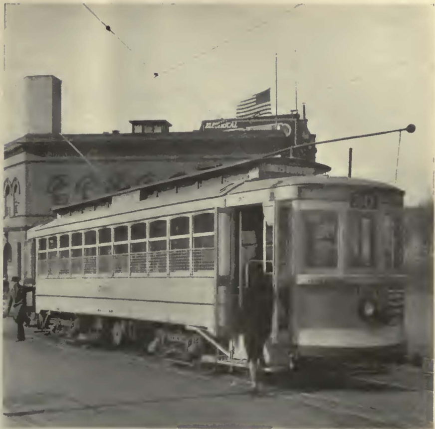
Remodeled car is arranged for one-man operation, entrance being at the front and exit at the rear by means of a treadle door
