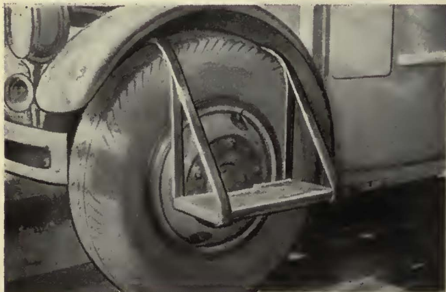
For making adjustments on motors of large buses a stand for the mechanic has been made in the shops of the Cleveland Railway
