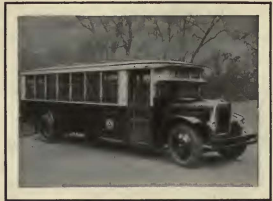
The Public Service Coördinated Transport of Newark, N. J., operates more than 1000 gas-electric buses equipped with G-E electric drive. In the design and manufacture of this type of equipment, General Electric has consistently led the field.
