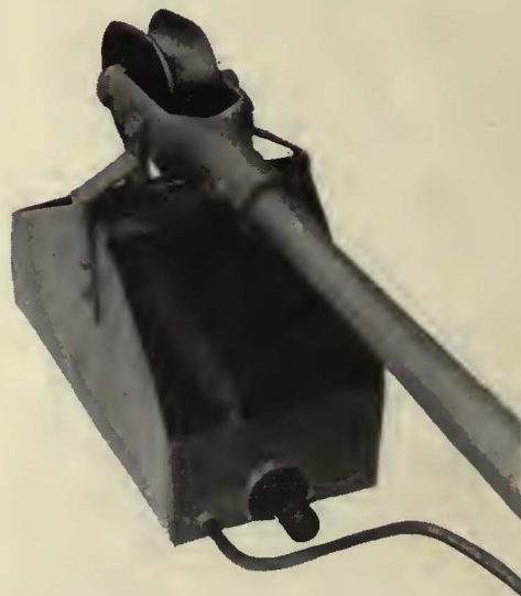
Apparatus used by Eastern Michigan Railways for applying lubricant to trolley wire, showing receptacle to catch excess liquid
