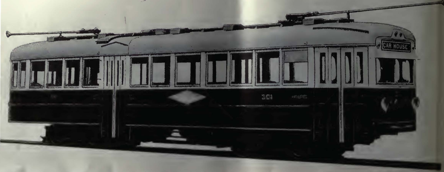
Car built by Cincinnati Car Company or United Traction Company of Albany. Alcoa Aluminum and its Alloys used for practically all metallic parts except wheels, axles, springs, bolts, rivets and nuts.
