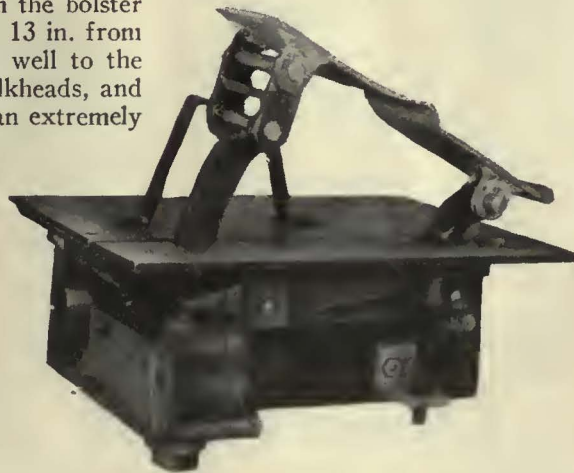
General Electric type C-523-A foot control, weighing only 38 lb., is used on the new Youngstown cars
