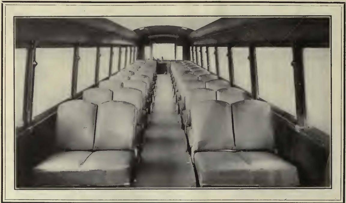
An interior view of one of 15 new light-weight cars recently completed by the Cincinnati Car Corporation for the West Penn Railways and the Monongahela & West Penn Railways. These cars featured Hale & Kilburn No. 392-A Walkover Seats with heat treated aluminum supporting framework and mechanism.
