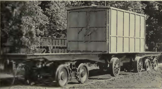
Fig. 10—Trailer of Bonner Railwagon system mounted on railway flat car
