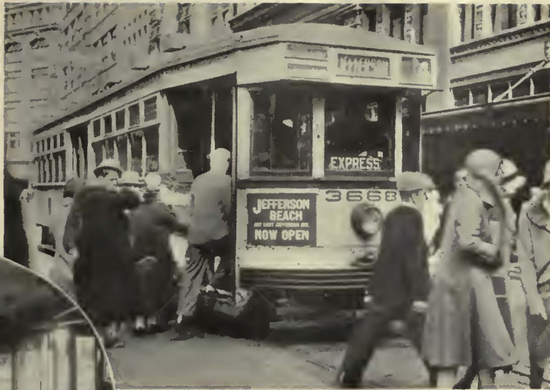
Wide doors and low steps reduce the loading time to a minimum on the Jefferson Avenue express line in Detroit
