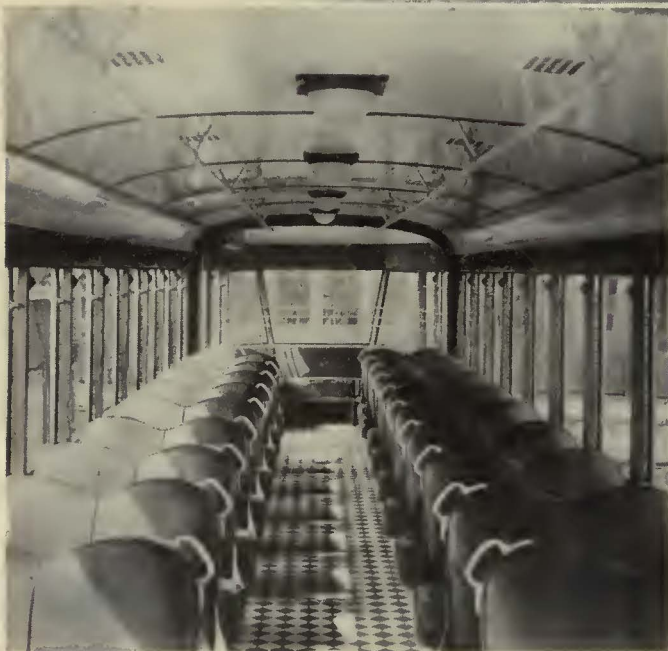
Top view—Two rows of dome lights, a reflecting ceiling and wide windows give ample artificial and natural light
