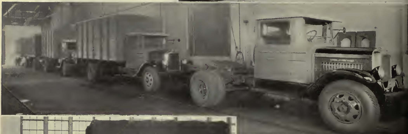
Fig. 5 (below)—Tractor, semi-trailer and four-wheel trailer equipment of the Northern Ohio Power, & Light Company. The truck with container body is used for both highway and pick-up and delivery service
