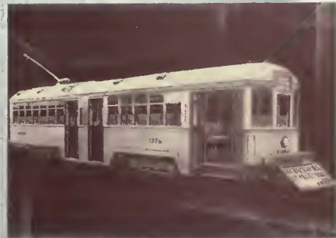
Built and operated by Cleveland Railway Co. In service Dec. 1926. Aluminum used on body, under-frame and trucks. Total weight of car 30,300 lbs. 6,647 lbs. of aluminum used. 12,901 lbs. dead-weight saved.
