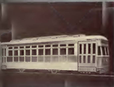
Built by J. G. Brill Co., for Third Avenue Rapid Transit System, N. Y. Aluminum used for body, under-frame and parts of the trucks. Total weight of car 27,000 lbs.
