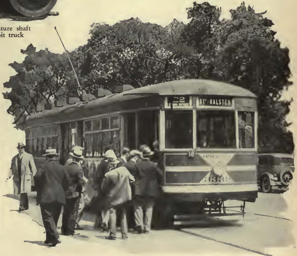
Latest Chicago Surface Lines car equipped with four 50-hp. motors for maintaining faster schedules
