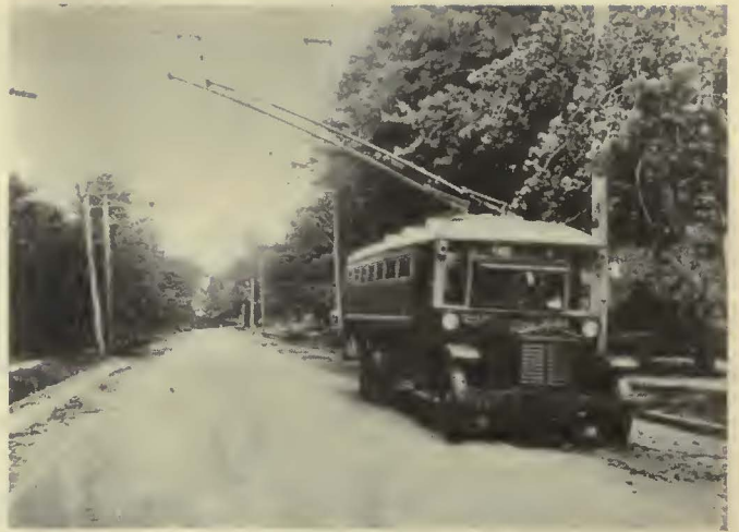
The old trackless trolley, with truck chassis, high body, projecting hood, heavy railway motors and hard rubber tires
