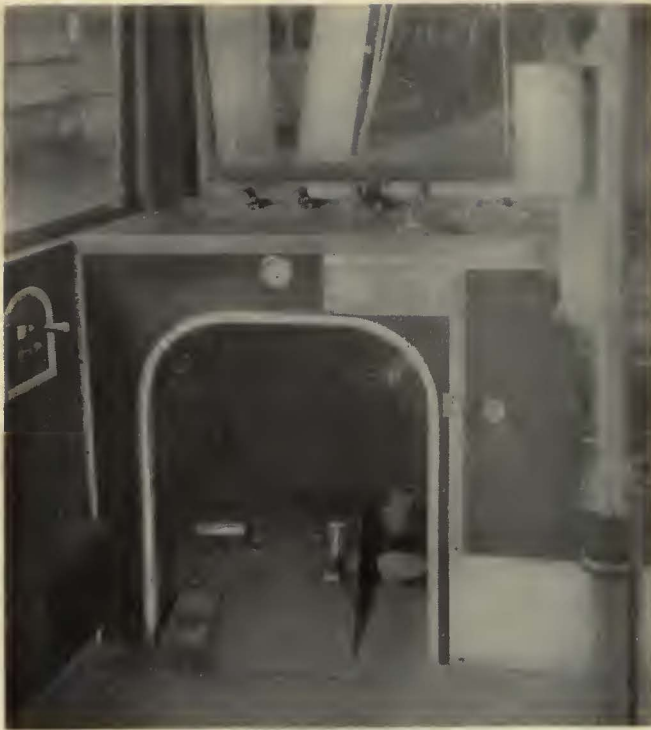
Foot control and convenient, plainly-marked auxiliary control handles simplify the duties of the motorman and make operation safer
