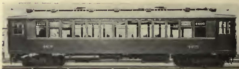
Recent type of Chicago Rapid Transit elevated car, using cross seats, an unusual practice for heavy service
