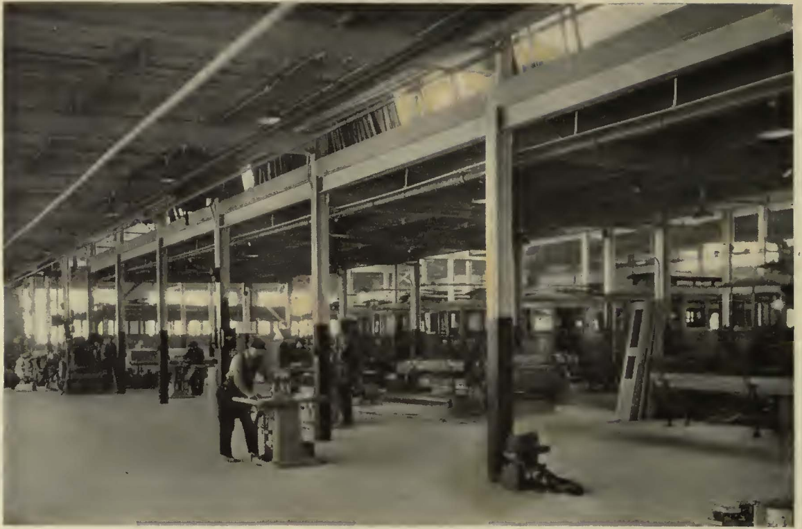
The mill room, located directly behind the body repair tracks. This arrangement was adopted for all the departments
