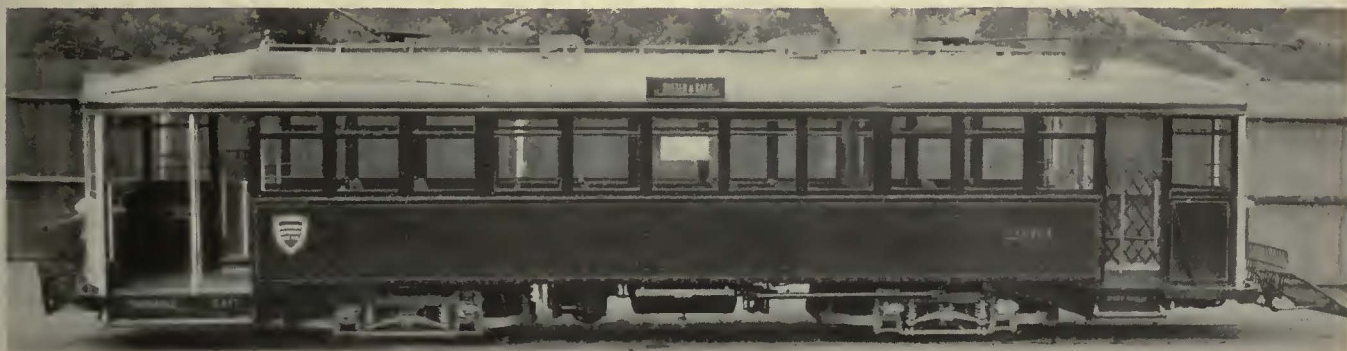
"Quiet" type car of the Market Street Railway, San Francisco, fitted with sound deadening materials under floor, rubber padding between car bolster and frame, leaded master gears, insulated gear boxes and quieted air compressors
