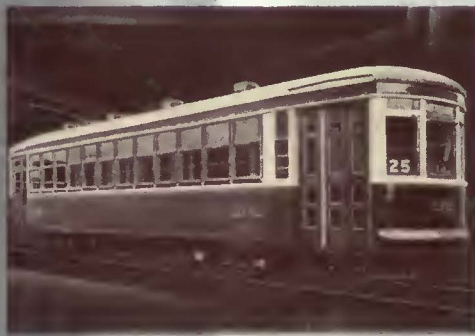
Built by Canadian Car and Foundry Co., for Montreal Tramways Ltd. In service 1927. Aluminum used for framing and exterior sheathing. Total weight of car 33,400 lbs. 2,275 lbs. of aluminum used. 3,700 lbs. of dead-weight saved.
