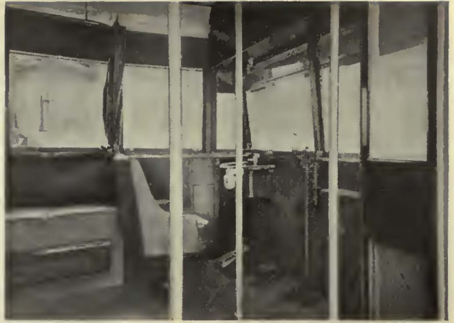
Mirrors, windshield wipers and wide vestibule windows aid the motorman in avoiding accidents
