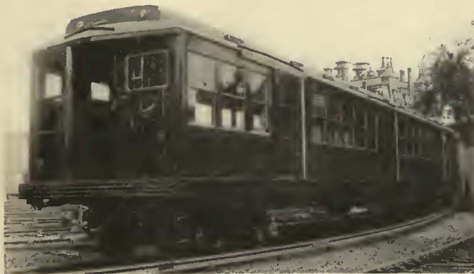
The doors on the new Cambridge cars are mounted on the outside rather than inside, and are electrically operated. The vertical white bands are the rubber door cushions
