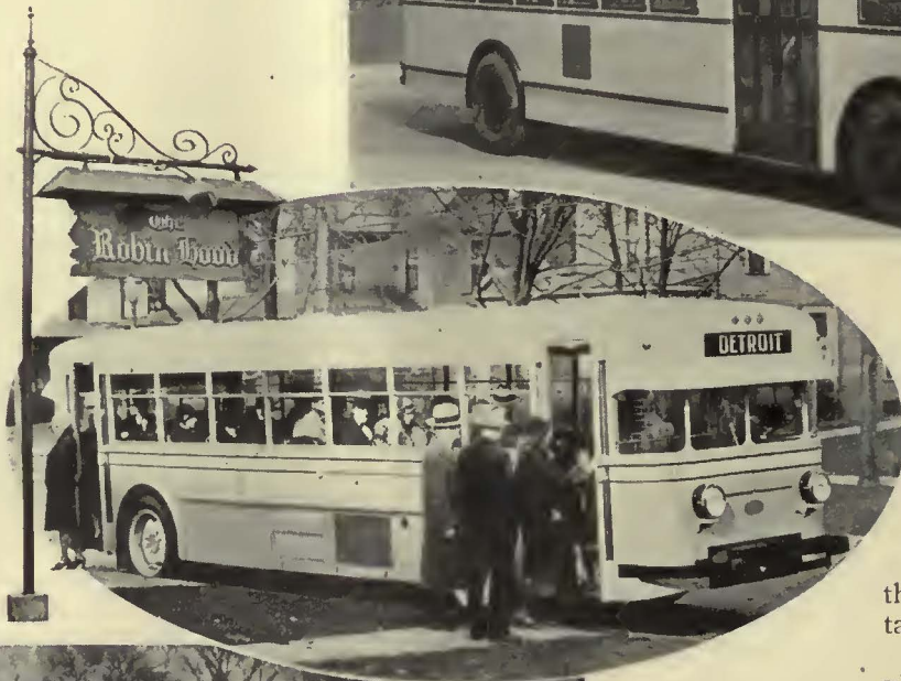
Larger capacity buses are one of the most important recent developments. For routes on which there is heavy passenger interchange, many are equipped with rear-exit doors
