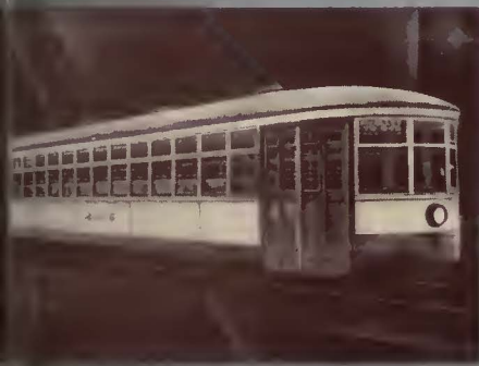
Built and operated by Twin City Rapid Transit Co. In service Dec. 1927. Aluminum used for sheets, posts and carlins. Total weight of car 27,670 lbs. 1,372 lbs. of aluminum used. 2,618 lbs. of dead-weight saved.
