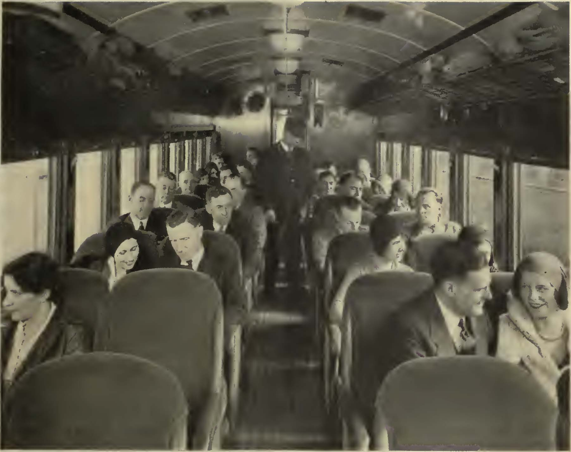
Plush-upholstered seats and a combination hot water and electric heating system, add to the comfort of passengers on the latest type of North Shore car. A thermometer and thermostat may be seen above the windows on the right
