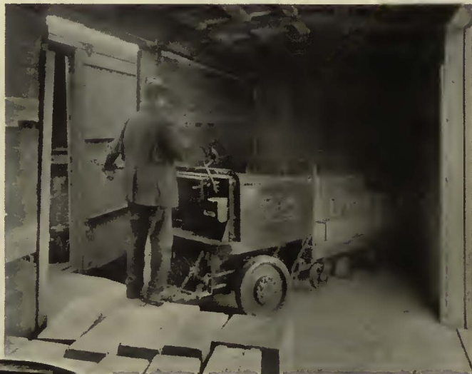
Fig. 14 — Elwell-Parker electric lift truck depositing skid in freight car
