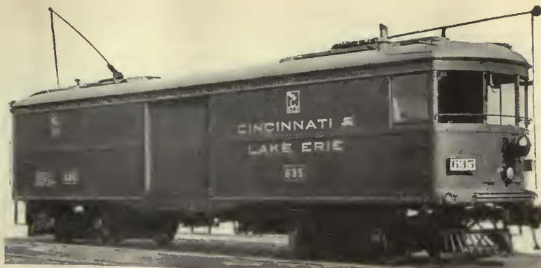
Fig. 2—Latest design of freight car, with a capacity of 80,000 lb., placed in service by the Cincinnati & Lake Erie Railroad. It is equipped with four 100-hp. motors and is capable of hauling twelve electric railway box car trailers at a speed of 45 m.p.h.
