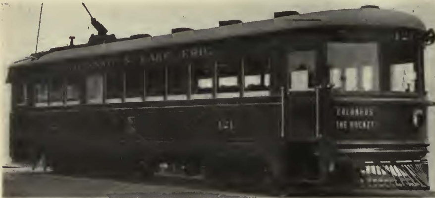
The new cars of the Cincinnati & Lake Erie Railroad are designed to make a maximum speed of 75 m.p.h.
