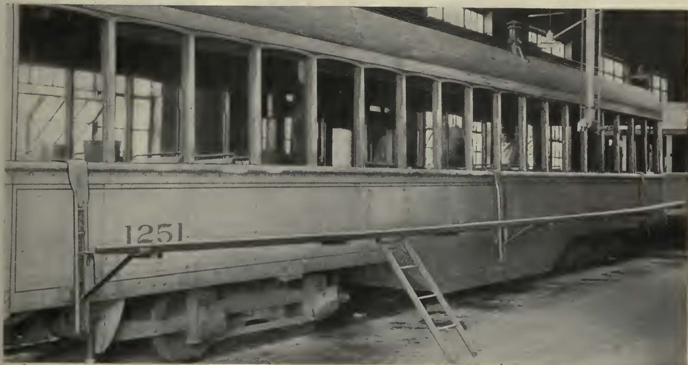
Brackets suspended from the windows support platform used in car washing or painting in the shops of the Cleveland Railway
