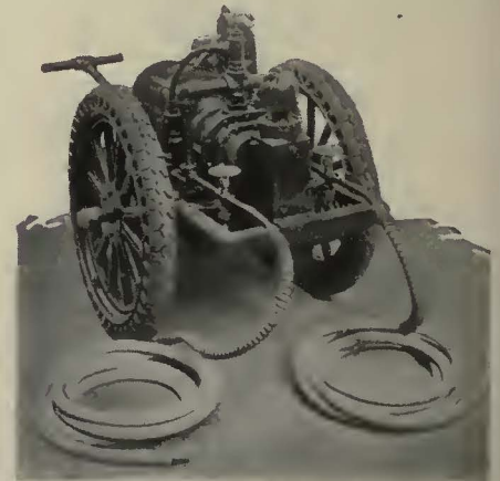
Compact preheater for making Thermit joints
