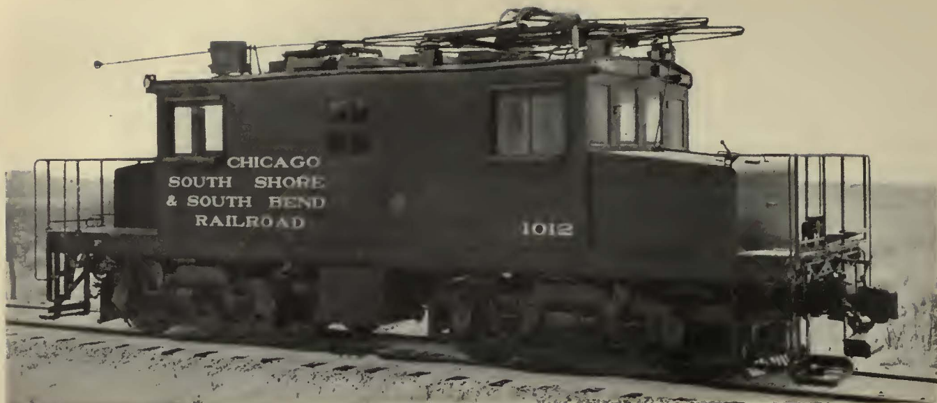
This 85-ton locomotive has been built for service on 1,500 volts and 600 volts, both trolley and third rail
