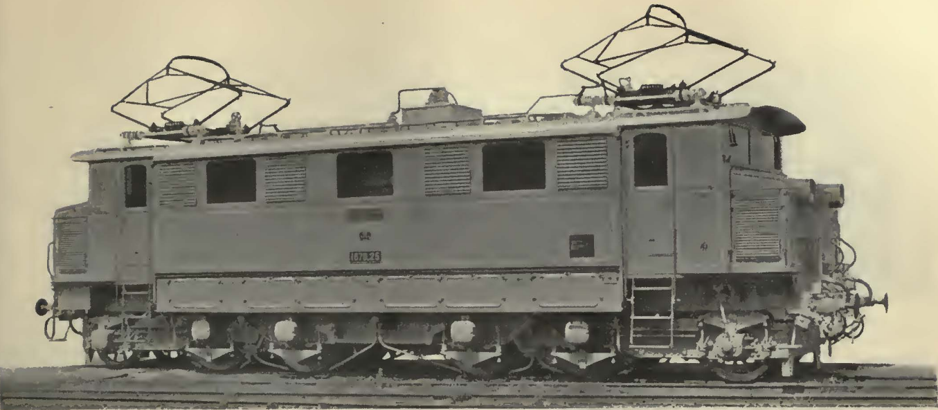
One of the new Austrian Federal Railways locomotives with vertical twin motors
