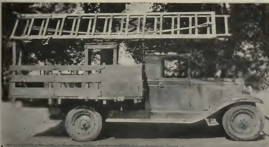
Telescoped sections of the ladder are easily carried on small motor truck
