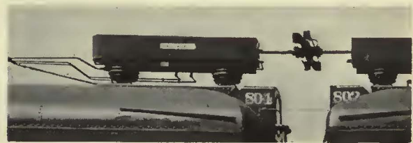
These new cars for the Reading will give service on suburban lines running out of Philadelphia. The inset below shows the 11,000-volt bus connector
