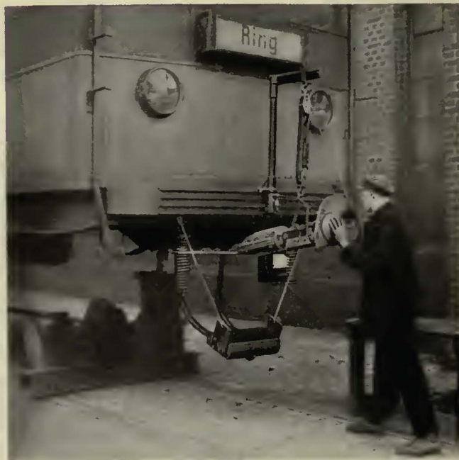
This convenient device makes removal and installation of automatic couplers easy in Hamburg
