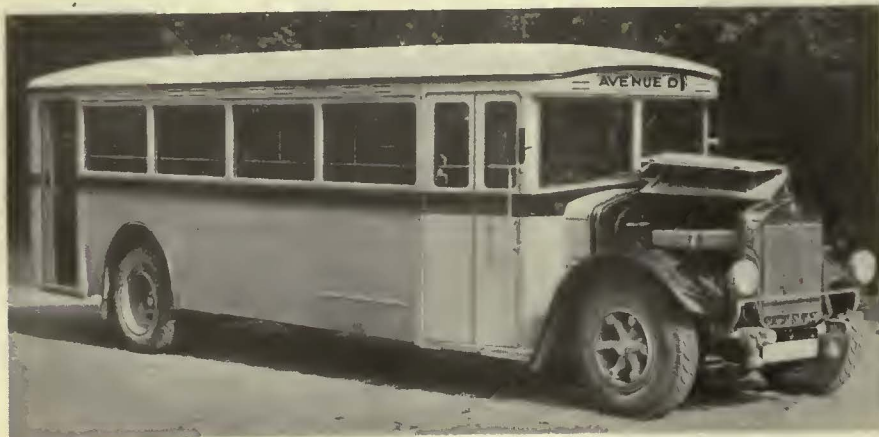
B.-M. T. recently tested this Diesel engine bus in a week of experimental operation
