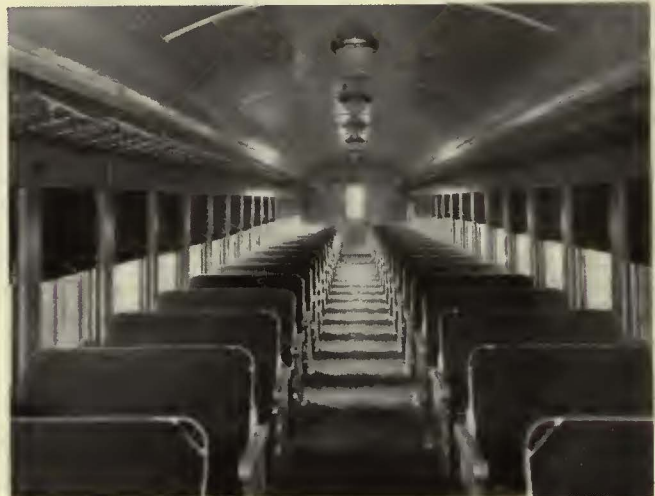
Right—The car interior is finished in three-tone gray, striped in blue and gold, with sanded nickel finish hardware. Brass window sash and Flexolith flooring also are features
