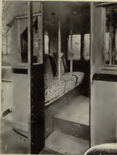
1—Rear compartment, showing the upholstered individual seats and stanchions with fare slots
