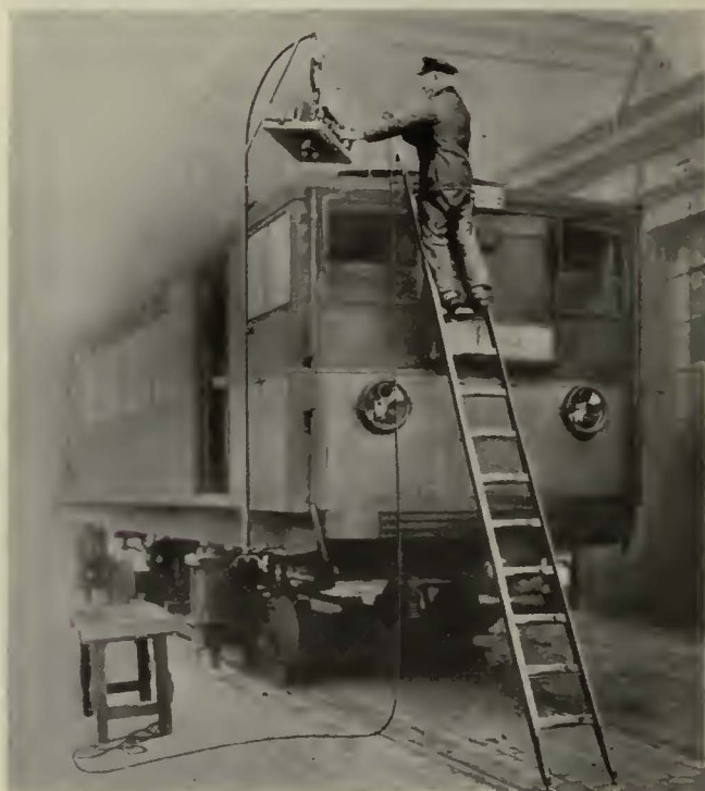
This light hand crane facilitates installation or removal of equipment on the car roofs in Hamburg
