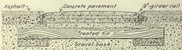
Cross-section of track as first built and as restored in 1914 and again in 1930
