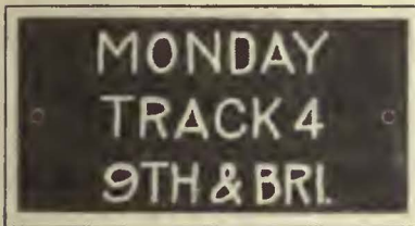
Tag on car shows when and where it is to be placed for inspection
