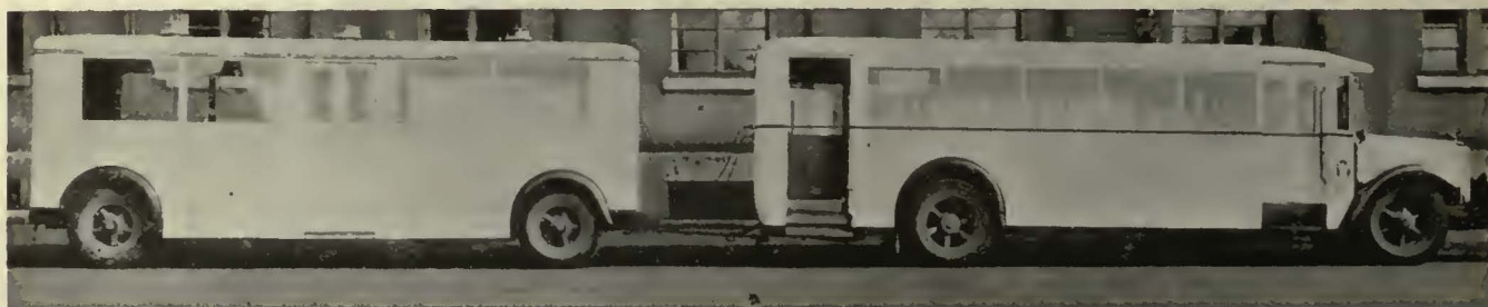
Street railways in Frankfort-on-the-Main, Germany, are carrying on experiments on Diesel buses with trailers. Fuel cost has been reduced from 0.75 to 0.12 pfenning per seat-kilometer through trailer use. Without trailer, the cost of fuel is 0.22 pfenning
