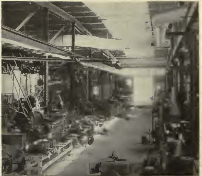
Armature shafts and commutators are being turned and bearings and pinions fitted in this section
