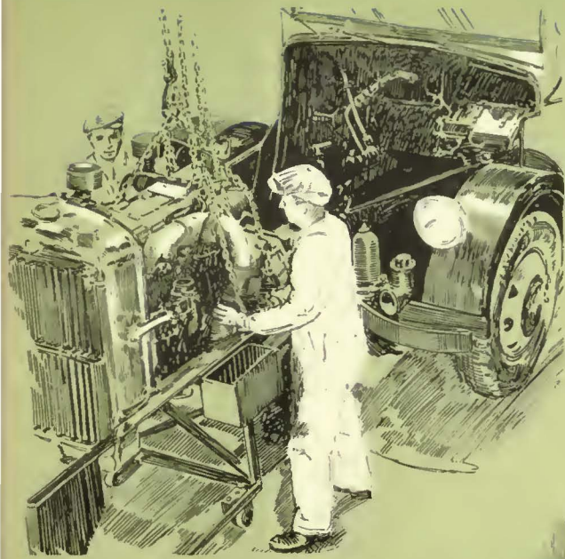
Without disturbing any adjustment or even removing the water from the radiator, two men can remove and replace the entire power plant assembly, including radiator, engine, clutch and transmission as a unit, in the same amount of time ordinarily required to replace a radiator.
