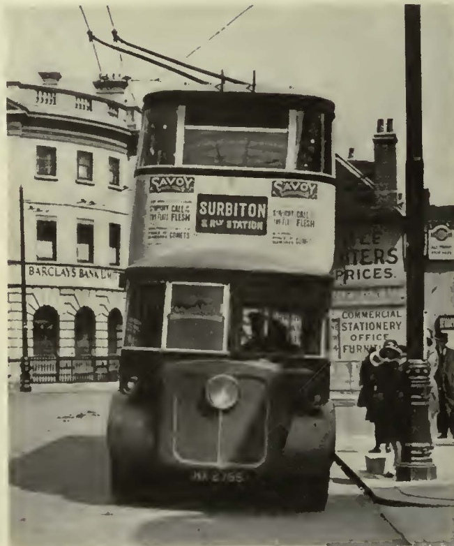
A special form of hood gives improved balance and proportion. These vehicles seat a total of 56 passengers
