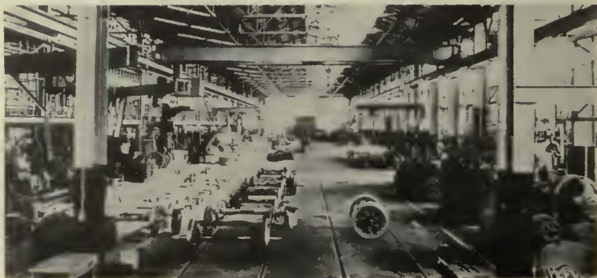
All machine tools in the wheel and axle shop are served by jib cranes or by the large overhead crane
