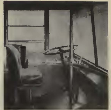
Driver's compartment showing control pedals and equipment cabinet
