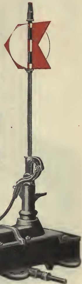
The adjustable oil buffer preventing return between successive pairs of wheels.
