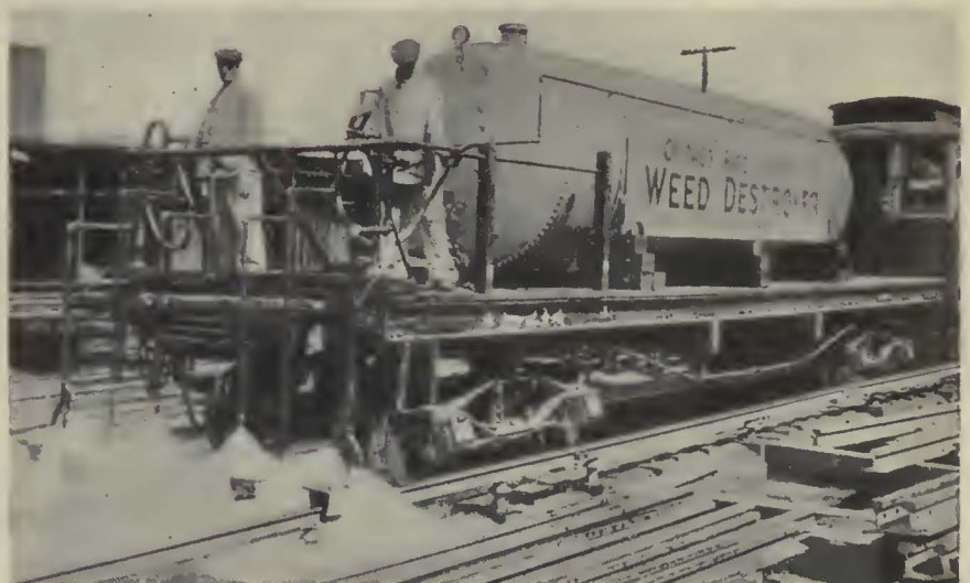
Tank car used by Chicago Rapid Transit Company for spraying acid solution to kill weeds along its right-of-way
