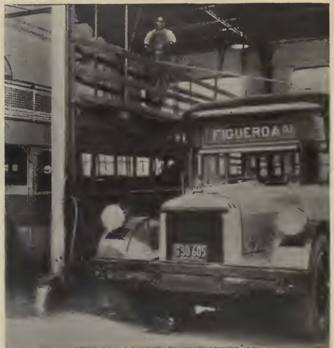
Tops are washed from a suspended platform with a long-handled water brush
