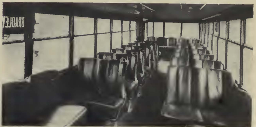
Leather upholstered seats, thermostatically controlled electric heaters, ample lighting and convenient arrangement of seats are provided in the interior
