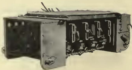
Modern demands have forced the controller off the platform in some of the latest cars. This unit switch control is typical of the designs adopted for use with a pedal
