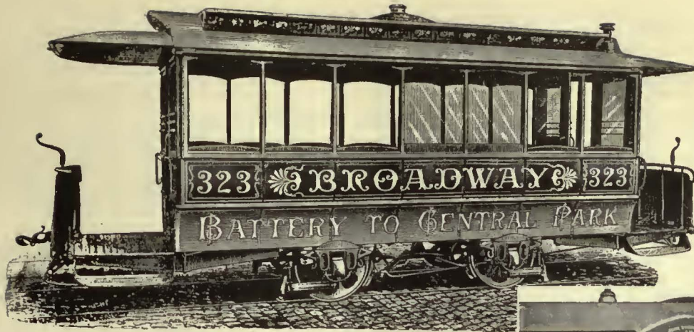
In the horse car days the journal boxes were mounted directly on the car sills, without trucks
