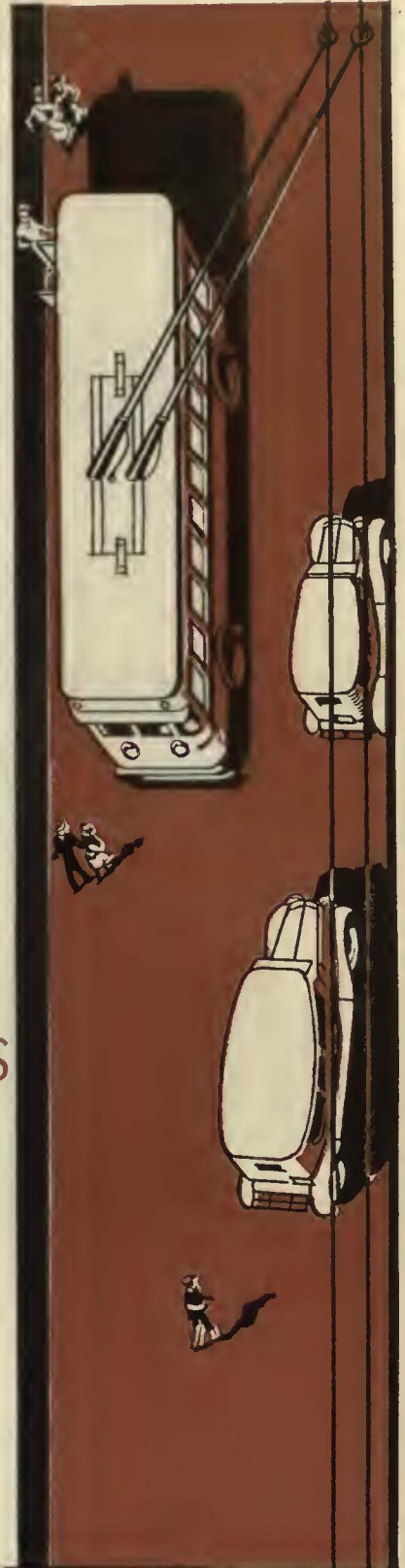
Note the off-center operation in the accompanying photograph and remember the contact wire guides your trolley wheel or shoe in trolley bus operation, not the car body as in the case of trolley car operation. With "PHONO" contact wire, the real benefit of high definite elastic limit is realized for the above purpose.
