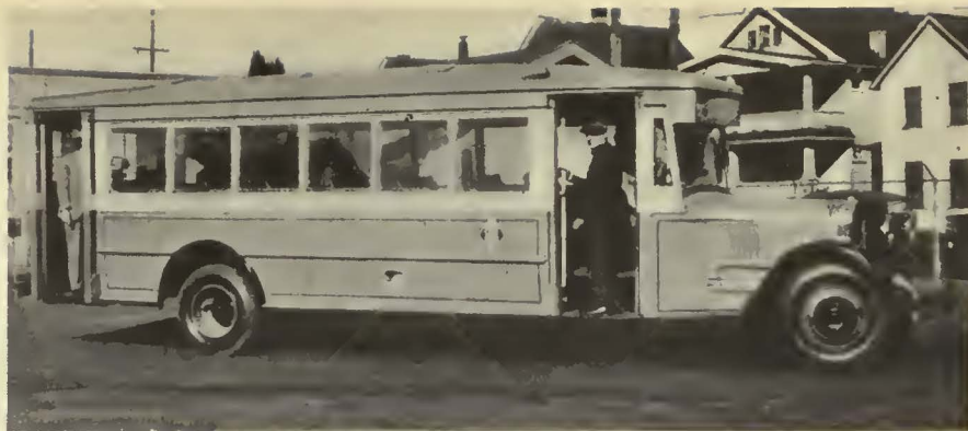
Steel bodies with automatic rear exit door were a new feature in 1928
