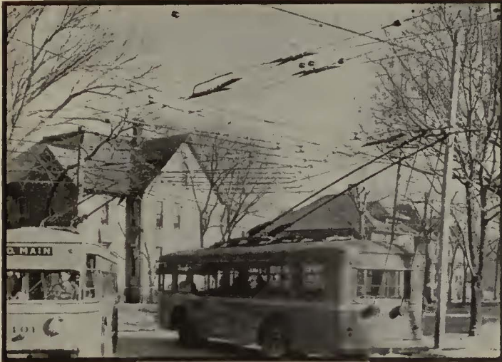
Note the off-center operation in the accompanying photograph and remember the contact wire guides your trolley wheel or shoe in trolley bus operation, not the car body as in the case of trolley car operation. With "PHONO" contact wire, the real benefit of high definite elastic limit is realized for the above purpose.
