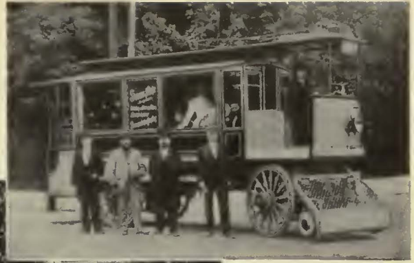
The first trolley bus in the world, built by Siemens and Halske, of Berlin, in 1899
