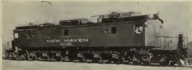
Most recent of the New Haven's passenger locomotives are these motor-generator units, which run either on single phase or direct current
