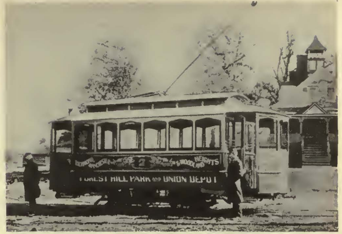
One of the early cars used at Richmond. The success of this installation in 1888 gave great impetus to the electrification of street railways
