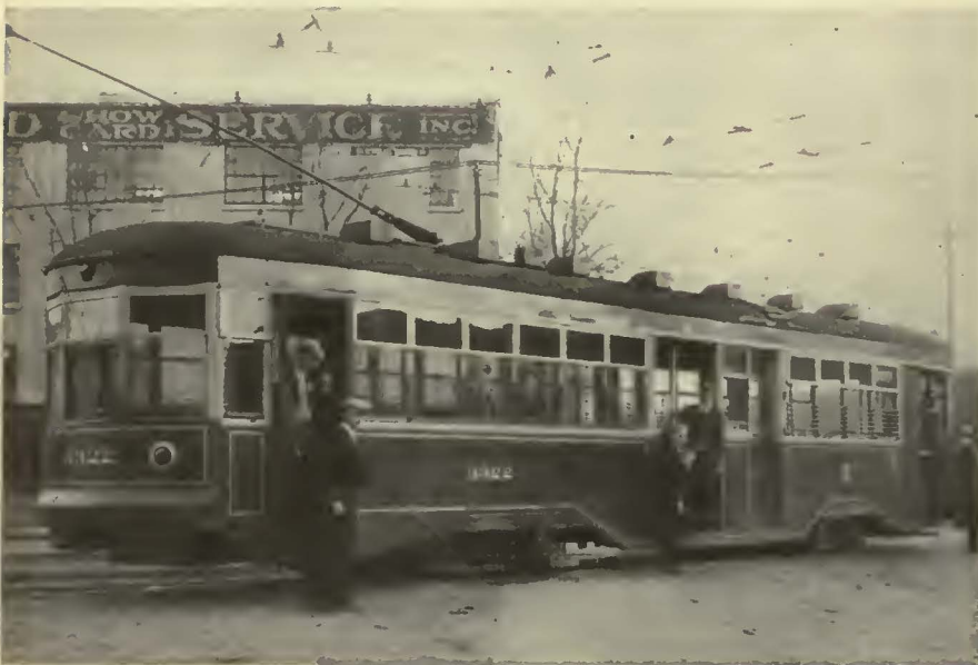
Modern large-capacity car with doors at front, center and rear is an efficient vehicle for handling mass transportation
