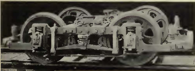
A standard short-wheelbase truck of the swinging bolster type of recent design
