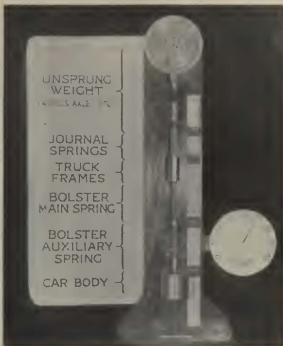
Simplified model to show spring action at various speeds. The wheel at the top corresponds to the car wheel. From it, a series of weights corresponding to the various elements of the car are suspended by springs corresponding to the car springs. When the wheel is rotated, the elements vibrate with the same characteristics as the elements of the car vibrate at various operating speeds Photos by William J. Ganz Company, New York Producers and distributors of talking pictures.
