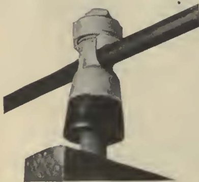
This Feeder Wire Insulator has a 3\frac{1}{2} -in. petticoat of Dirigo insulating compound, extending below the metal parts. Into this Dirigo is molded a 1-in. pin-hole to fit standard wood pins. The saddle on which the cable bears is curved to conform with the droop of the wire to avoid damage to heavy cables. The 1\frac{1}{2} -in. seat accommodates standard 500,000-circ. mil weatherproof cable. Manufacturer: Ohio Brass Company, Mansfield, Ohio.
