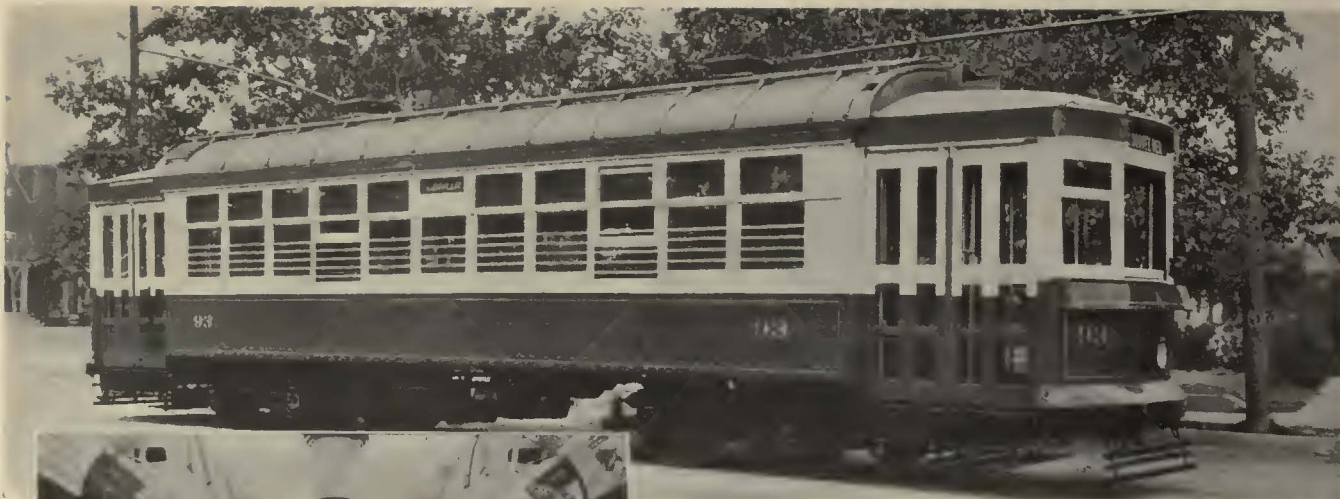
El Paso's rebuilt car for service on the Juarez line, operating across the Mexican border
