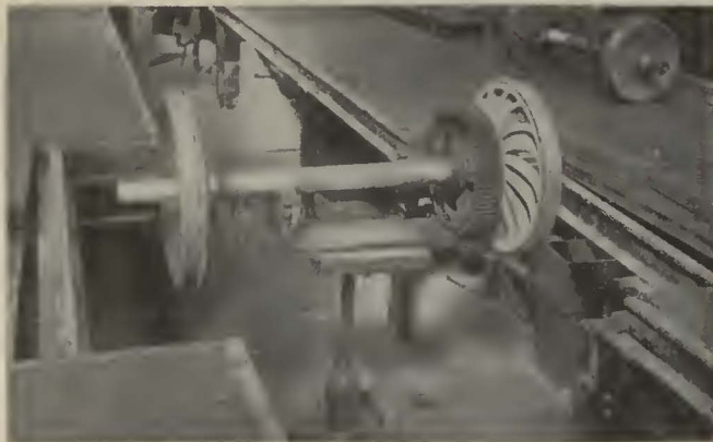
Hydraulic jack used by the Toronto Transportation Commission to remove wheels with safety
