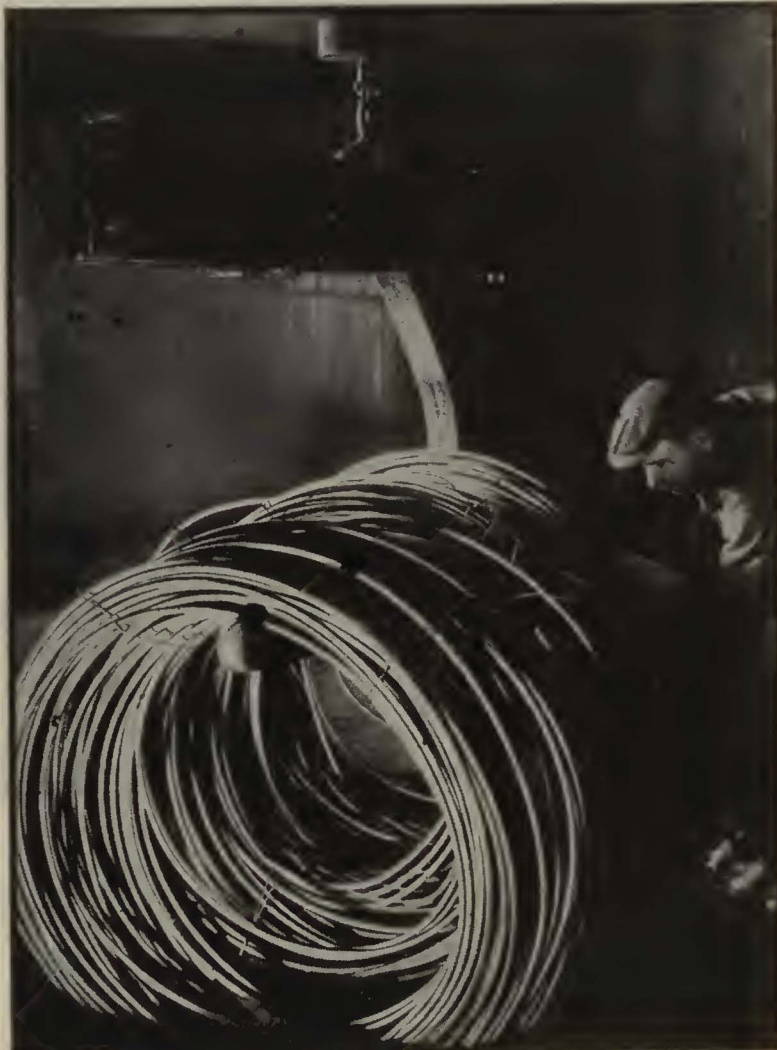
A pickling room operation in an R B & W plant, in which scale and dirt are removed from raw materials.
