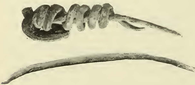
NO. 0 COPPER WIRES EATEN AWAY BY ELECTROLYSIS.
