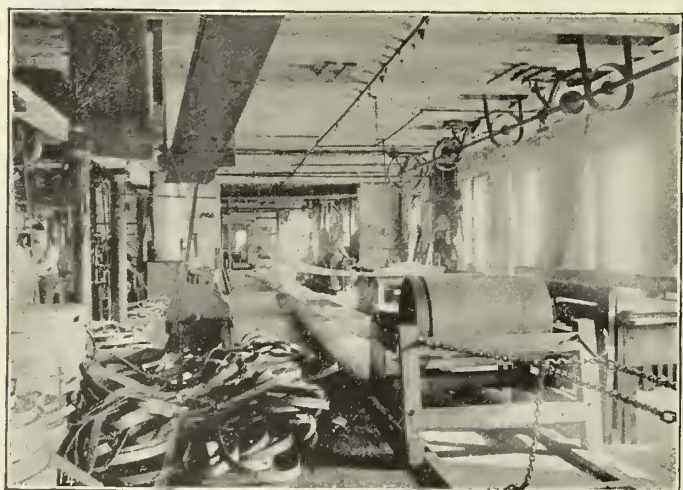
FIG. 12.—CEMENTING AND PRESSING A FORTY-EIGHT INCH BELT.
