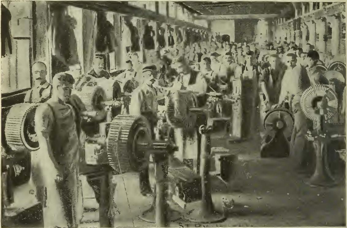
FIG. 8.—WINDING W. P. MOTOR ARMATURES.
