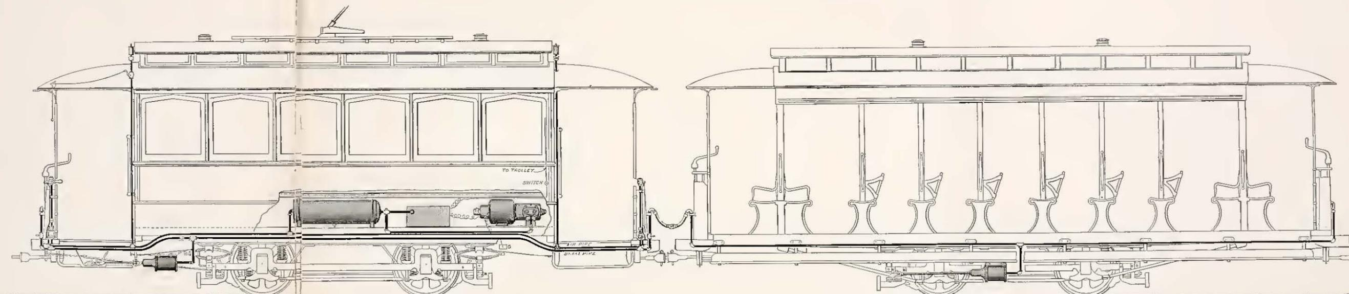
PLAN AND ELEVATION, SHOWING THE AIR BRAKE EQUIPMENT FOR STREET CARS,
