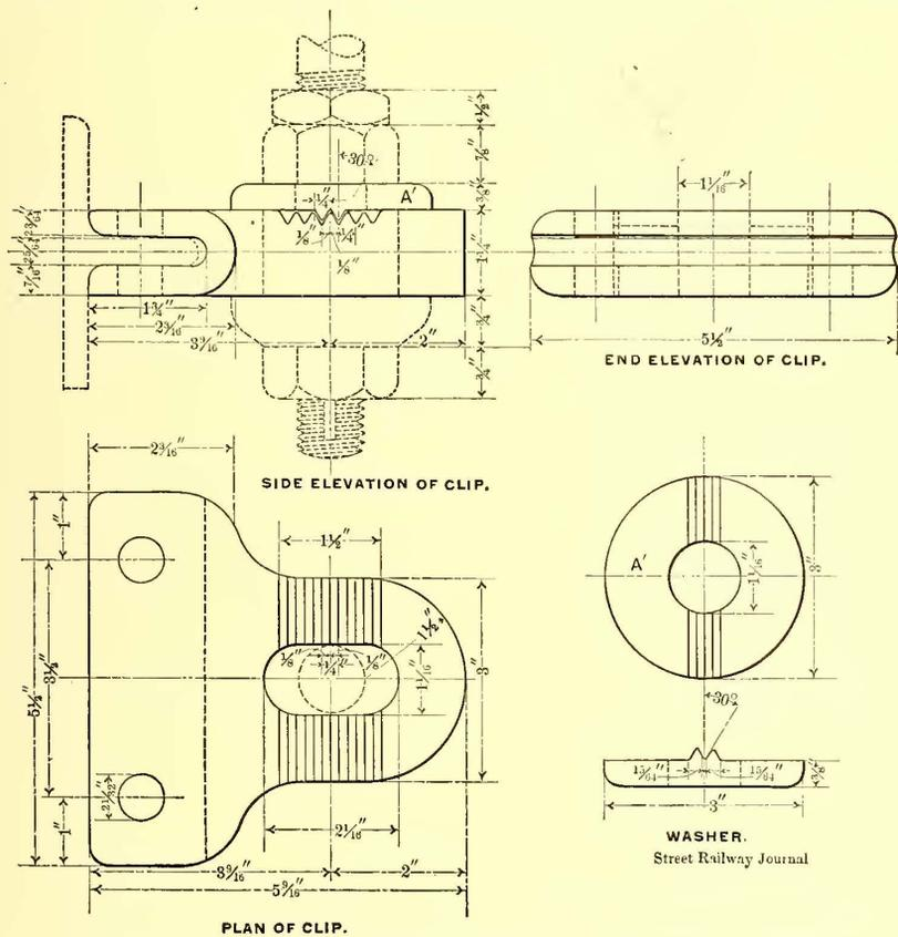
FIG. 1.—NEW CLIP AND EAR FOR UNDERGROUND CONDUIT.
