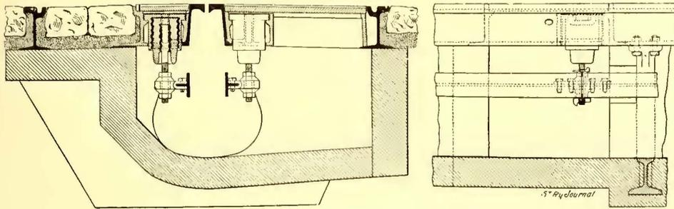
FIG. 5.—CROSS AND LONGITUDINAL SECTION OF CONDUIT AT INSULATOR.
