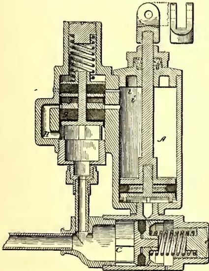
FIG. 3.—SECTION OF AUTOMATIC GOVERNOR FOR COMPRESSOR.
