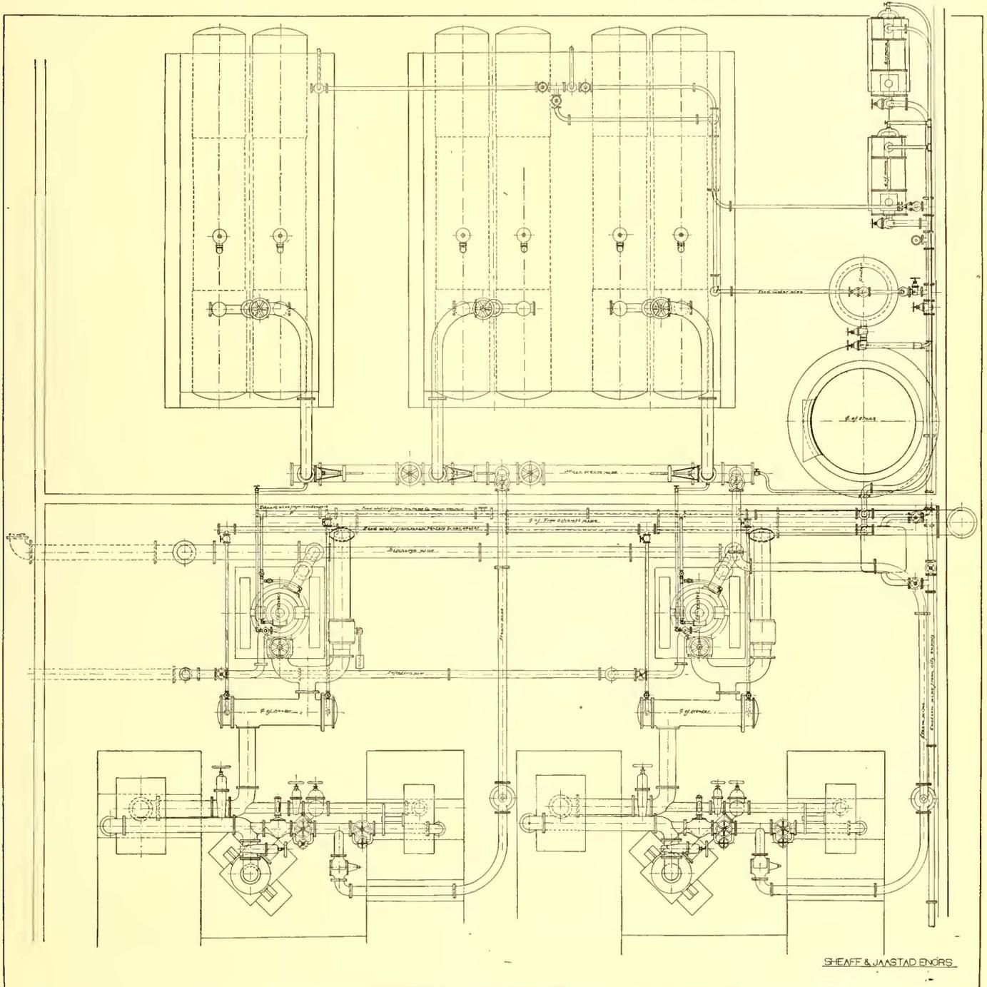
FIG. 3.—PLAN OF STATION, SHOWING PIPING.
