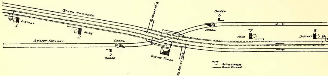
PLAN OF STREET AND STEAM RAILWAY CROSSING PROTECTED BY INTERLOCKING SIGNALS.
