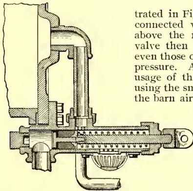
FIG. 4.—SECTION OF GRADUATING VALVE.
