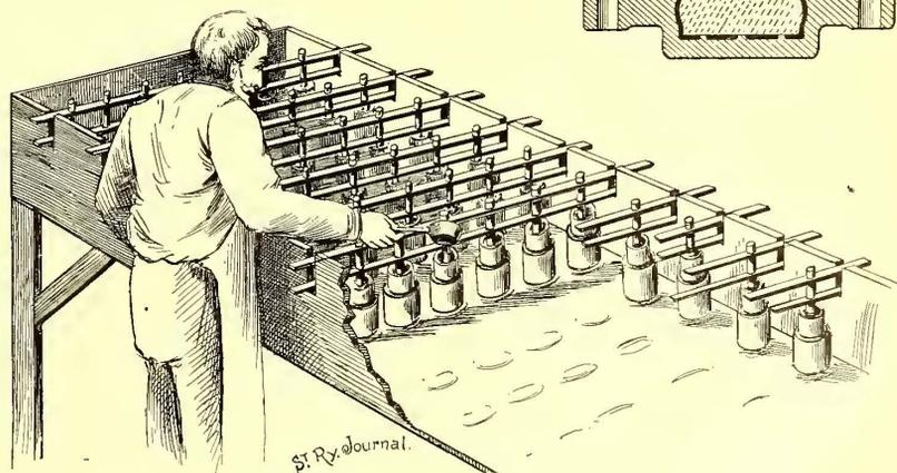
FIG. 2.—METHOD OF ASSEMBLING INSULATORS.
