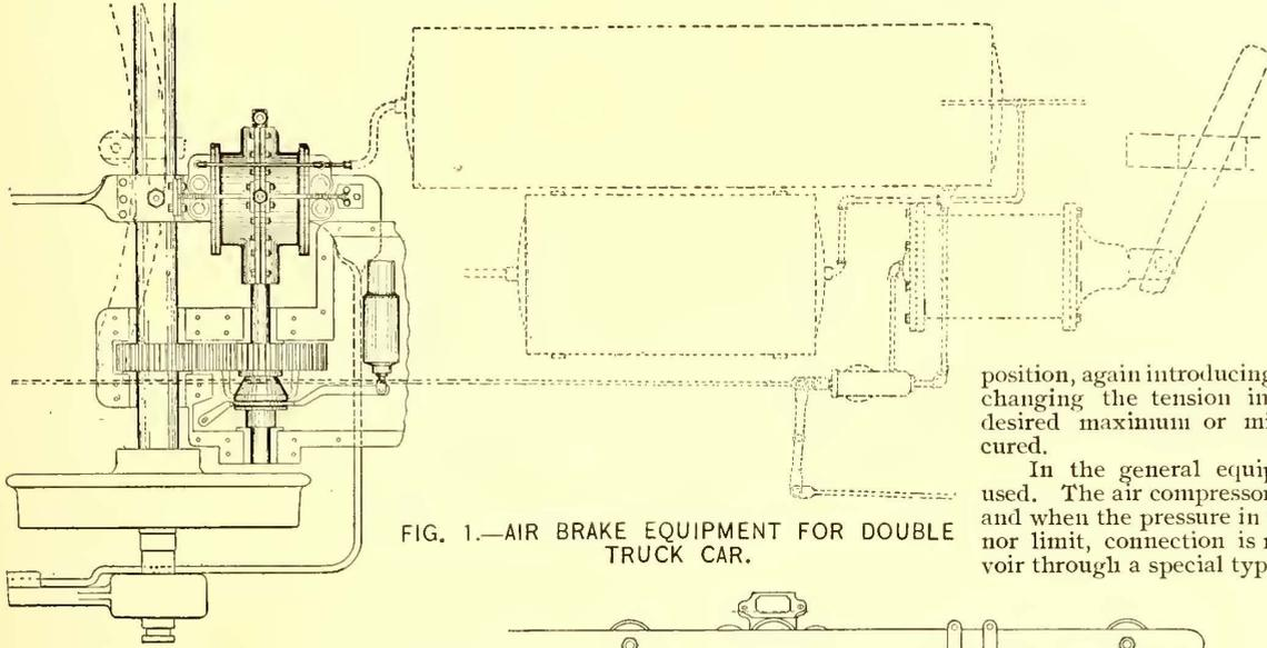
FIG. 1.—AIR BRAKE EQUIPMENT FOR DOUBLE TRUCK CAR.
