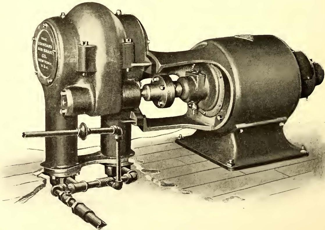
FIG. 2.—ELECTRIC COMPRESSOR.
