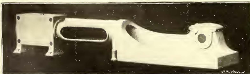
FIG. 53.—THE REYNOLDS-CORLISS "1890 FRAME"
