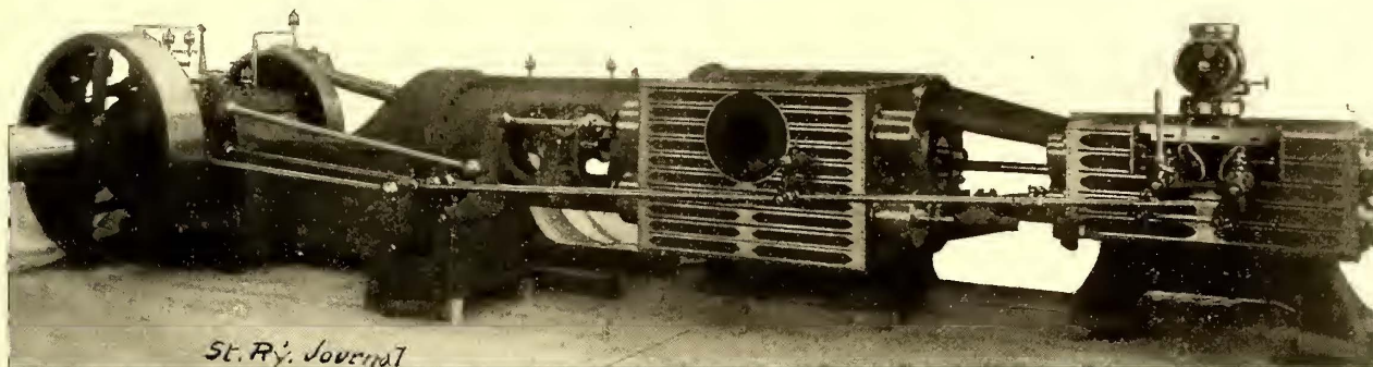
FIG. 76.—FITCHBURG 20 IN. AND 38 IN. X 42 IN. TANDEM COMPOUND ENGINE
