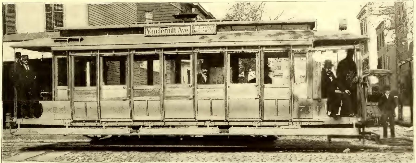
FIG. 11.—VIEW OF CONVERTIBLE CAR SHOWING DOORS CLOSED
