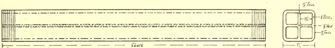
SIDE ELEVATION AND SECTION OF PIPE
