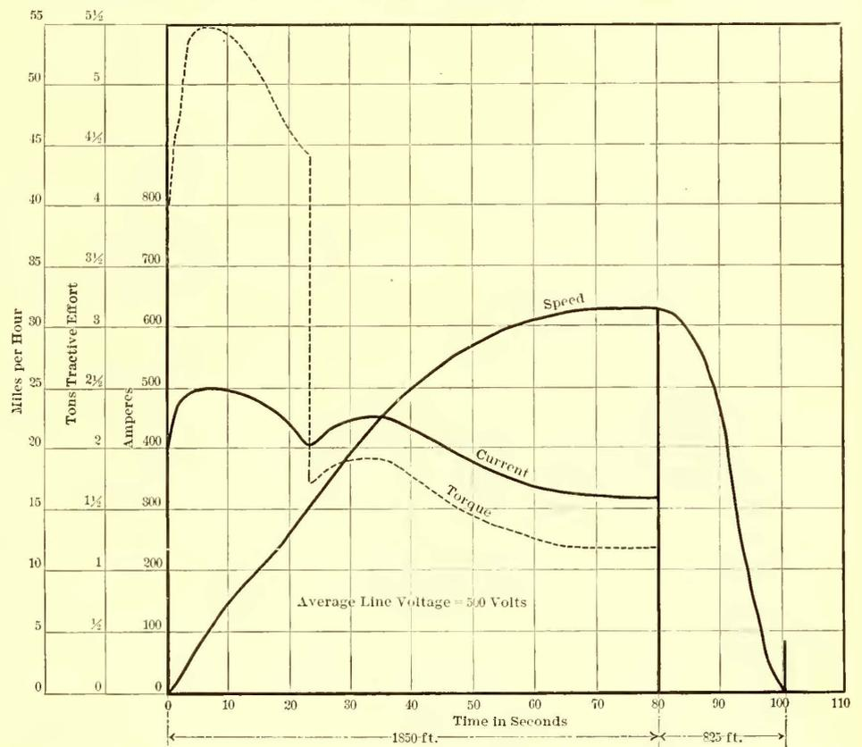
FIG. 8—CURVES SHOWING ACCELERATION AND CURRENT CONSUMPTION OF LAKE ST. (CHICAGO) 5 CAR, 90 TON TRAIN—2 150 H. P. MOTORS
