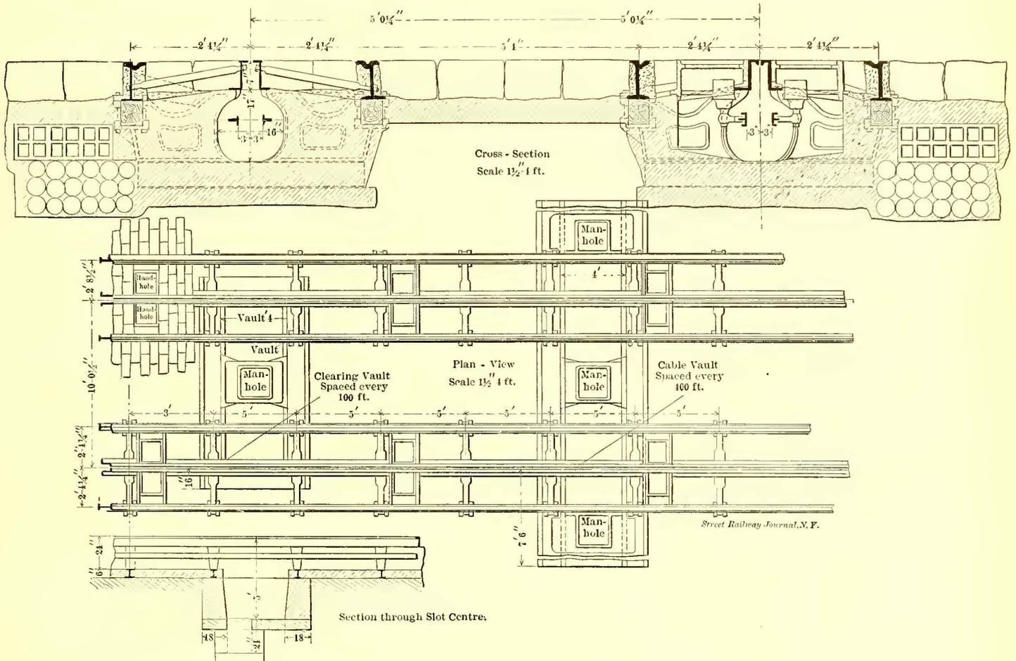
FIG. 1.—PLAN AND SECTIONS OF STANDARD NEW CONSTRUCTION, THIRD AVENUE RAILWAY
