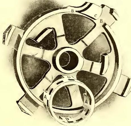
FIG. 3.—WHEEL FRAME AND ACTUATING RING
