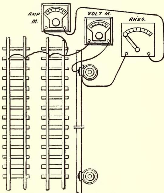
FIG. 4.—DIAGRAM OF CONNECTIONS FOR MEASURING FLOW FROM RAIL TO PIPE
