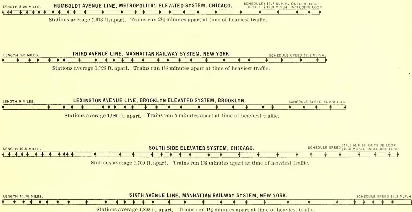
FIG. 3—CHARACTERISTICS OF FIVE HEAVY TRAFFIC ELEVATED LINES IN NEW YORK AND CHICAGO
