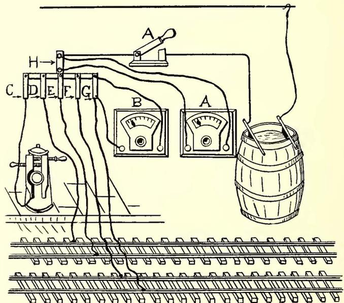
FIG. 5.—DIAGRAM OF CONNECTIONS FOR MEASURING RELATIVE VALUE OF RETURNS
