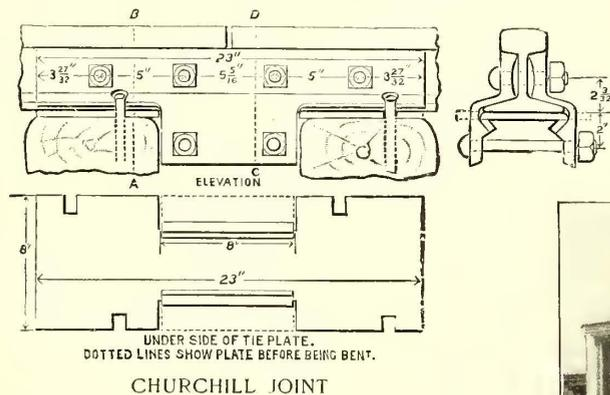
turned edges of the engaging portions of the base plate, so that when the two lower truss bolts are tightened up, there is formed a wedge adjustment which insures the keeping of the parts always in close contact, making them practically one with the rail, giving it great security and strength.
