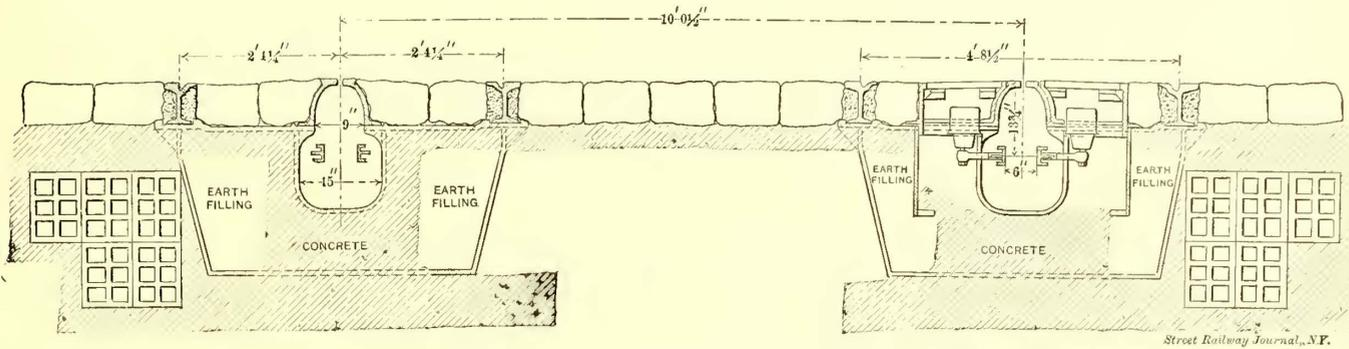
FIG. 6.—SECTION THROUGH ROADBED ON THIRD AVENUE
