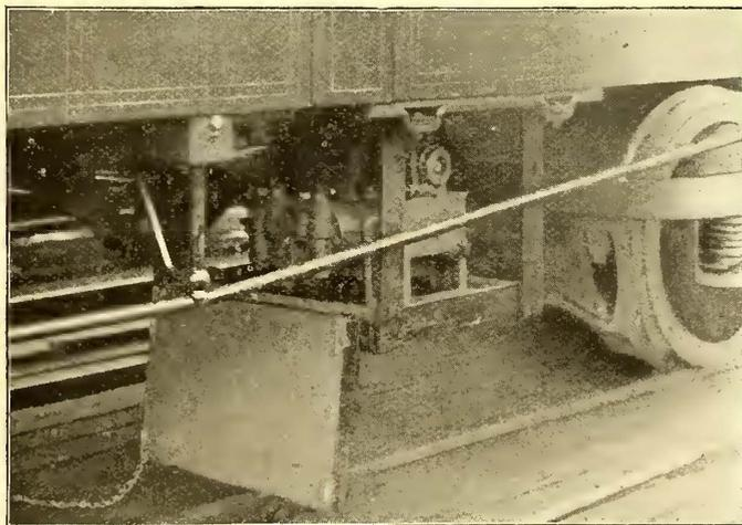
ELECTRIC MOTOR AIR COMPRESSOR
