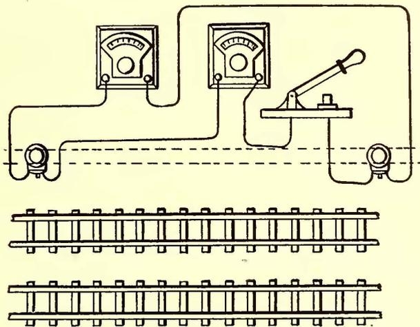
FIG. 3.—DIAGRAM OF CONNECTIONS FOR MEASURING FLOW IN PIPES
