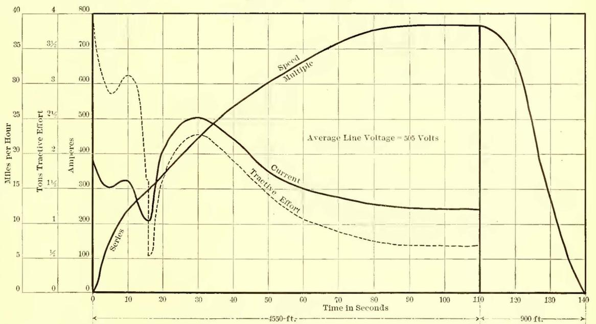
FIG. 9—CURVES SHOWING ACCELERATION AND CURRENT CONSUMPTION OF LAKE ST. (CHICAGO) 3 CAR, 58 TON TRAIN—2 150 H. P. MOTORS
