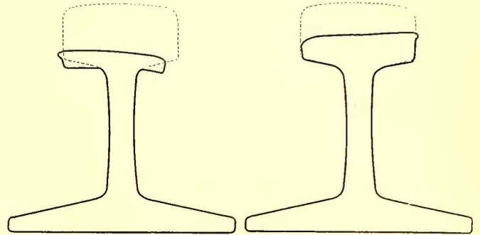
FIG. 2.—RAILS ON CURVE AFTER ONE YEAR'S SERVICE
