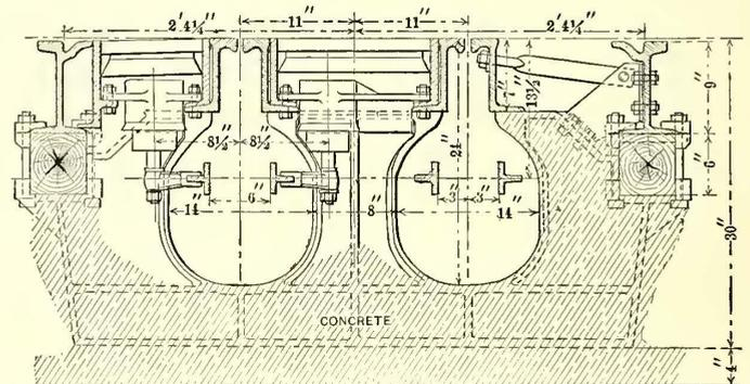
FIG. 3.—SECTION OF DUPLEX CONSTRUCTION WHERE TWO COMPANIES OPERATE OVER SAME TRACK
