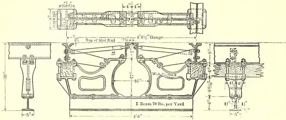
FIG. 2.—STANDARD YOKE, NEW CONSTRUCTION
