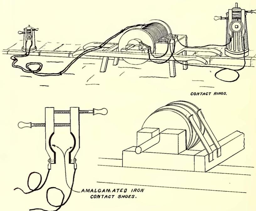
FIG. 2.—APPARATUS FOR MEASURING CURRENT FLOW IN WATER PIPES
