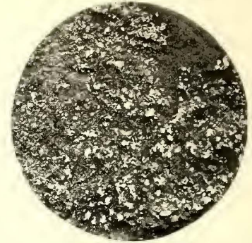
FIG. 5.—FRACTURE OF HAMMERED IRON AXLE
