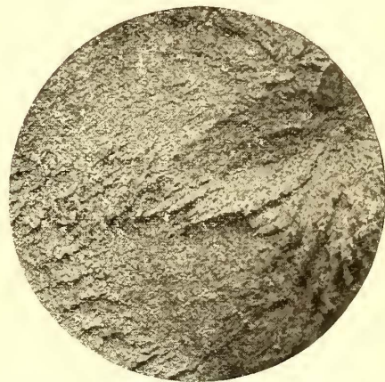
FIG. 1.—FRACTURE OF FINE STEEL AXLE
