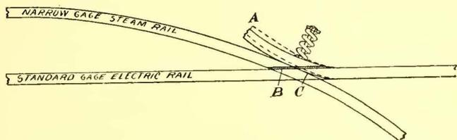
FIG. 2.—SPRING FROG AT CROSSING OF STEAM AND ELECTRIC RAILWAY
