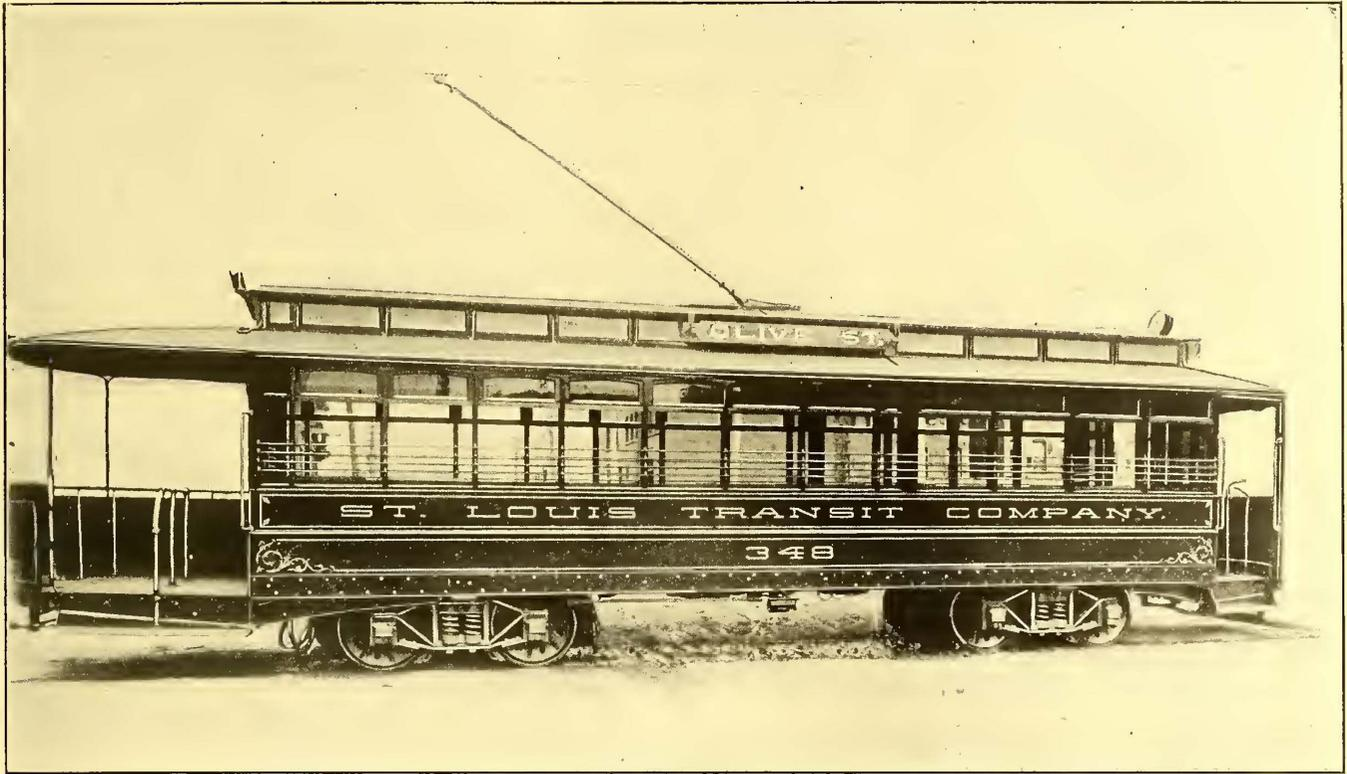
FIG. 20.—NEW SPLICED CAR WITH DETROIT PLATFORM
