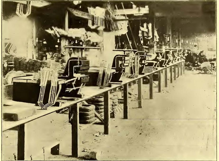
FIG. 10.—PRESSES FOR INSULATING ARMATURE COILS
