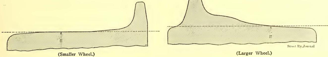
FIG. 1.—WEAR PRODUCED WHEN WHEELS ARE OF DIFFERENT DIAMETER
