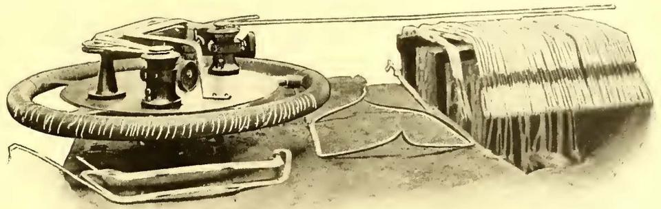
FIG. 5.—ARMATURE COIL WINDER FOR G. E. 800 MOTOR
