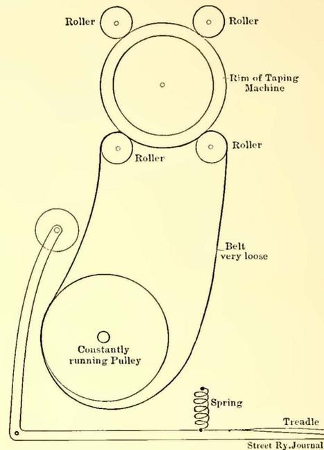
FIG. 8.—DEVICE FOR DRIVING TAPING MACHINE
