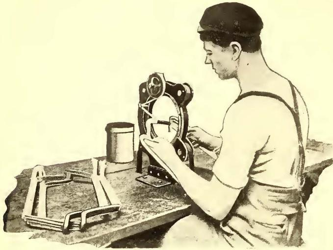
FIG. 7.—COIL TAPING MACHINE
