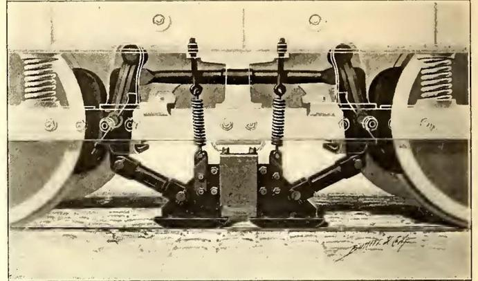
FIG. 2.—VIEW SHOWING METHOD OF ATTACHING BRAKE, TO CAR
