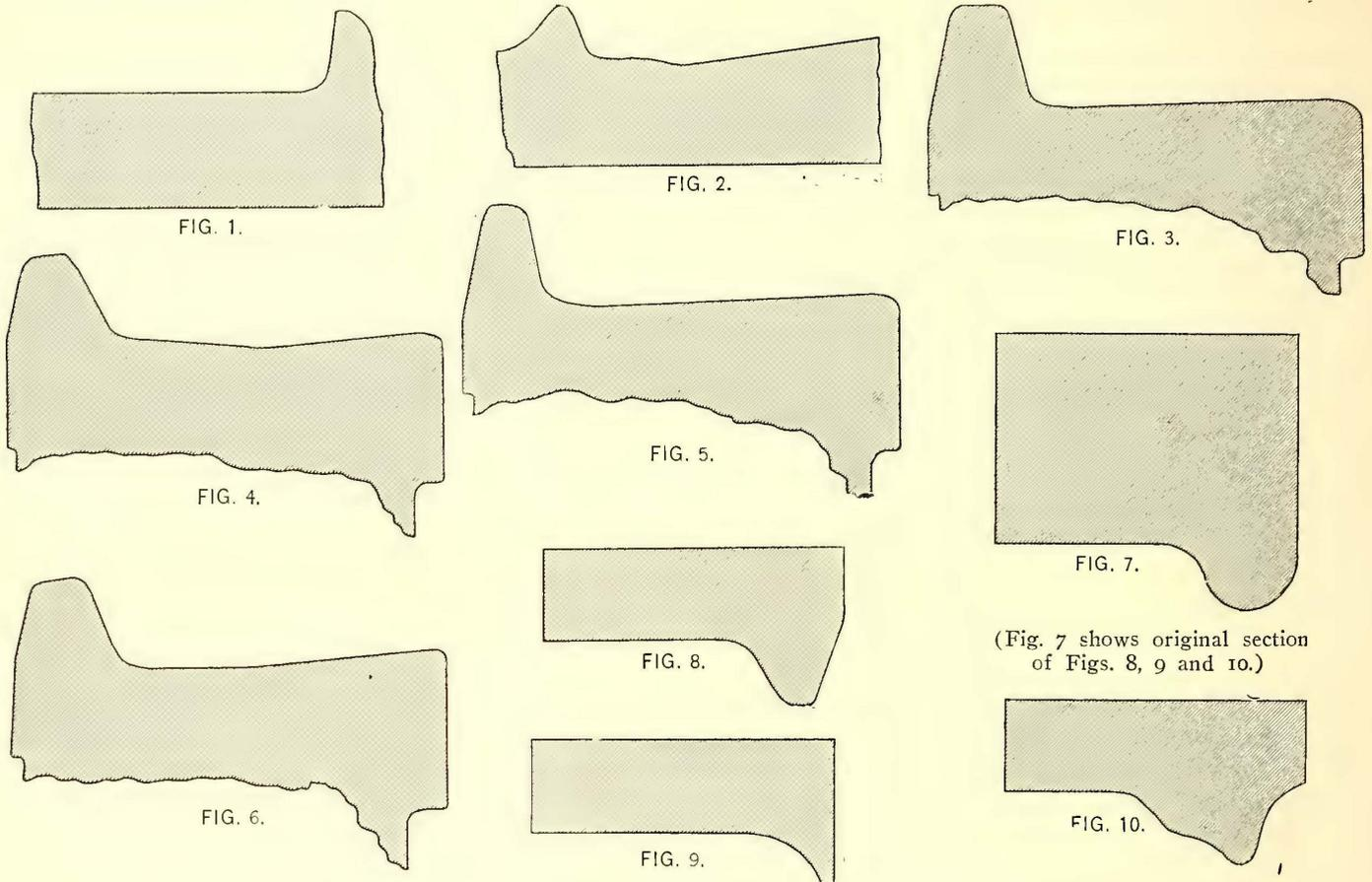
SECTIONS OF STEEL WHEELS WORN ON FLANGE OR TREAD
