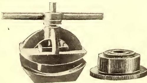
FIG. 13.—FIELD COIL PRESS
