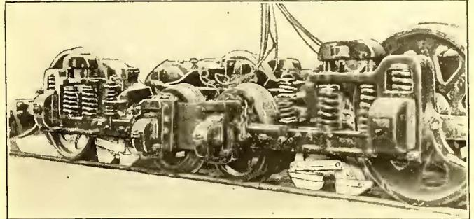
FIG. 5.—METHOD OF ATTACHMENT TO A MAXIMUM TRACTION TRUCK
