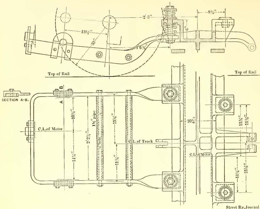
FIG. 24.—MOTOR SUSPENSION OF DOUBLE TRUCK
