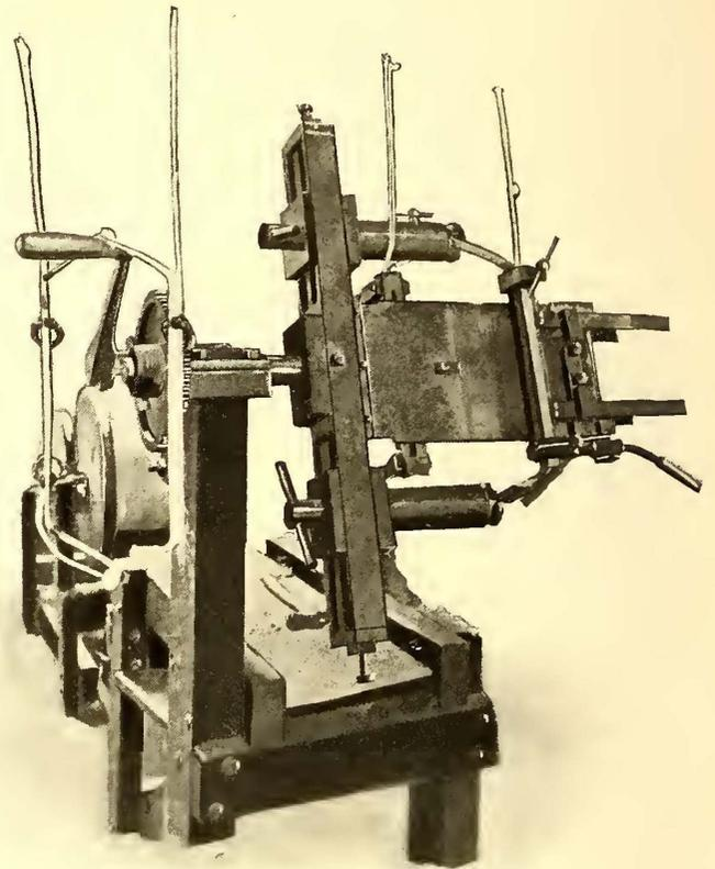
FIG. 2.—ARMATURE COIL WINDER FOR G. E. 57 AND OTHER MOTORS, COIL SPREAD READY TO TAKE OUT
