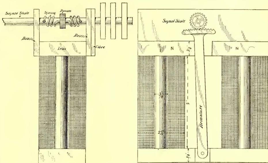
FIG. 1.—SECTIONS OF ELECTRO MAGNET USED IN OPERATING BLOCK SIGNAL SYSTEM
