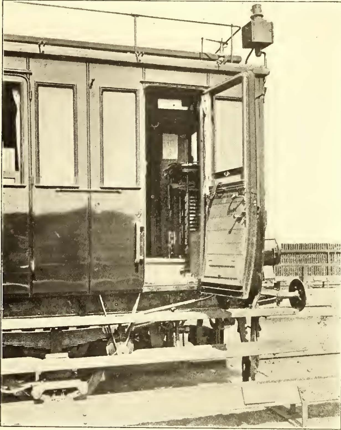
FRONT OF CAR, SHOWING CONTROLLER, WANNSEE RAILWAY
