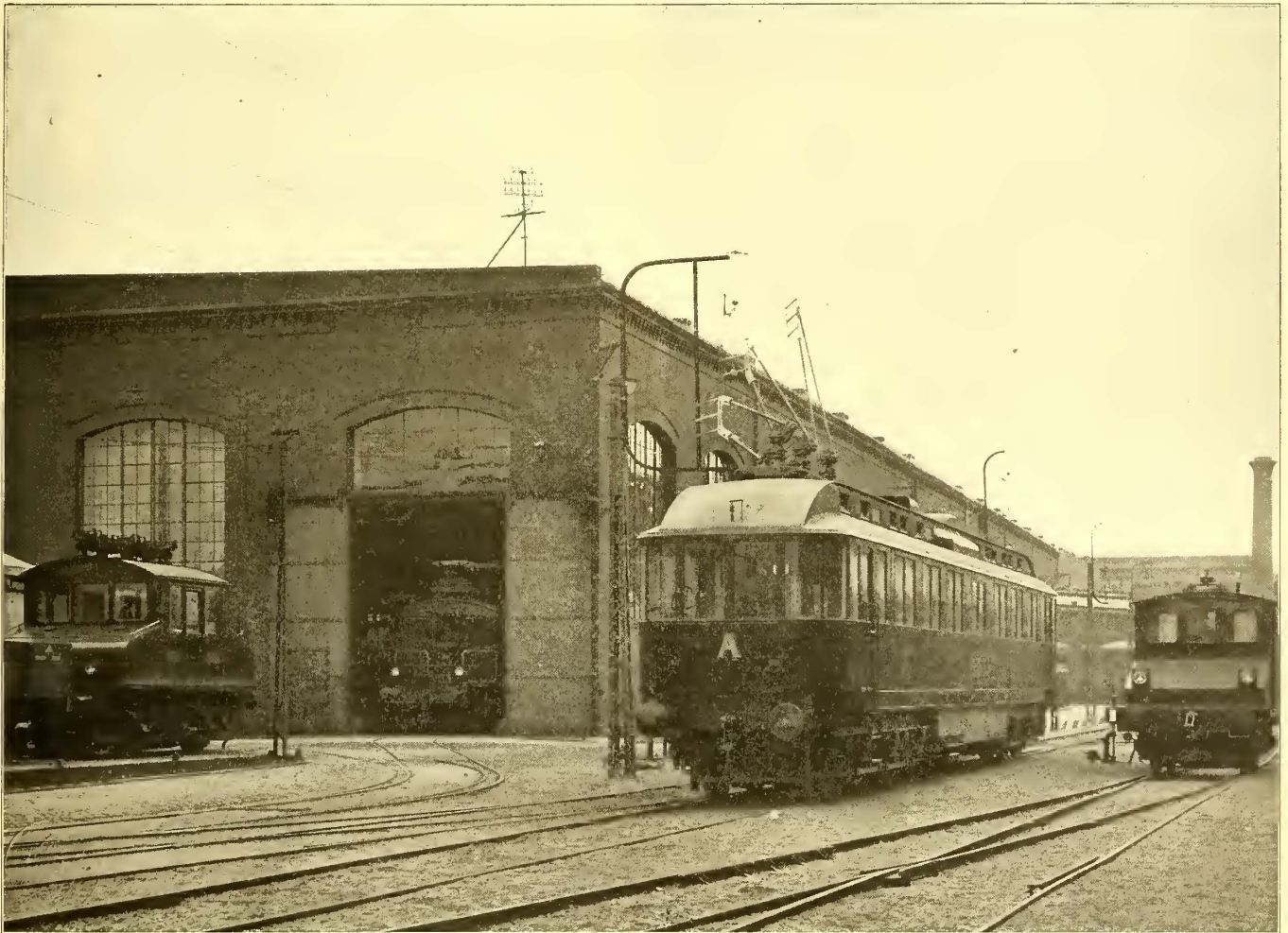
FIG. 1.—EXPERIMENTAL CAR BUILT TO OPERATE AT 125 MILES PER HOUR ON THE BERLIN-ZOSSEN LINE
