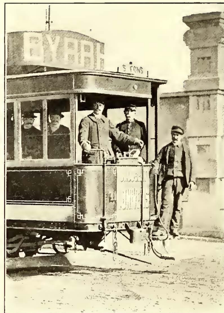
FIG. 16.—A FRENCH CAR WITH STEPS AT THE END CORNER OF PLATFORM
