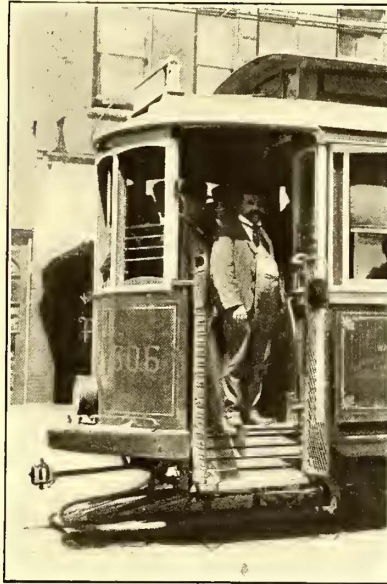
FIG. 14.—BOTH DOORS AND GATES OPERATED BY MOTORMAN
