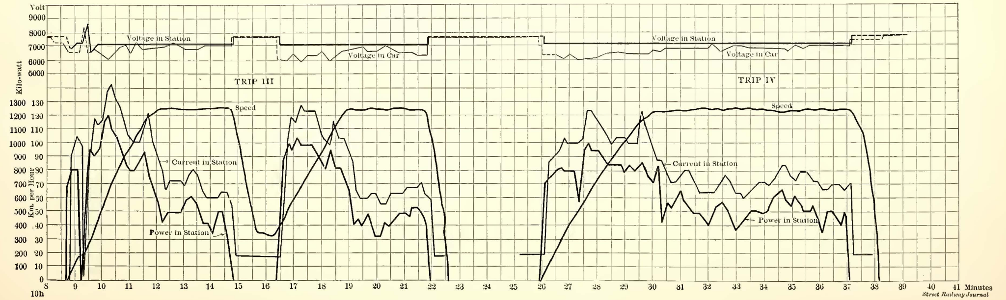
FIG. 4.—SPEED, CURRENT, VOLTAGE AND POWER OF CAR "S" IN ZOSSEN TESTS
