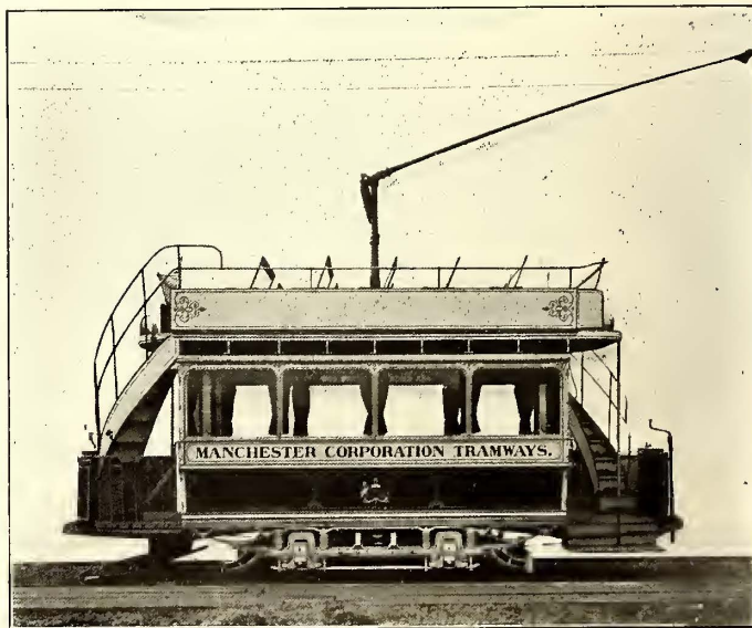
FIGS. 4 AND 5 — STANDARD SINGLE TRUCK CARS, MANCHESTER CORPORATION
