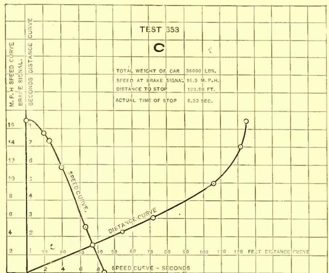
FIG. 1.—TIME AND DISTANCE CURVES FOR EMERGENCY STOPS
