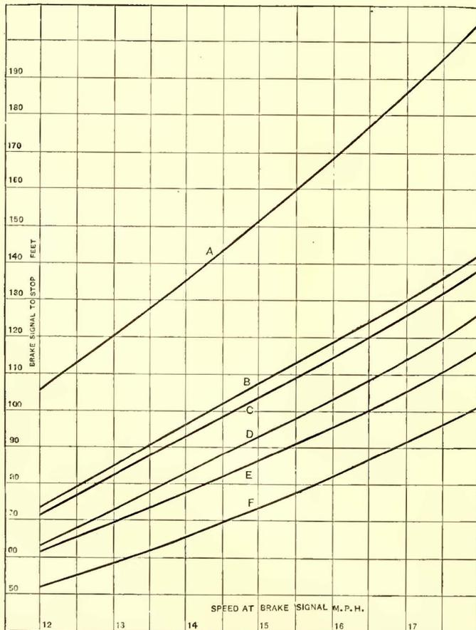
FIG. 2.—COMPARISON CURVES FOR EMERGENCY STOPS
