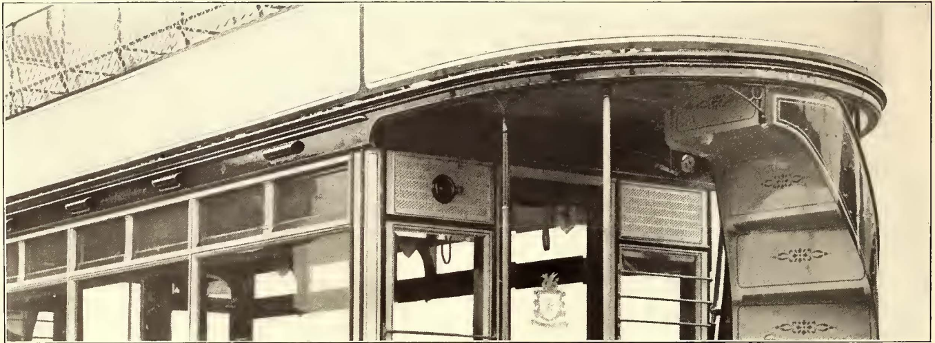
FIG. 1.—UPPER PART OF CAR, SHOWING HINGED WINDOW
